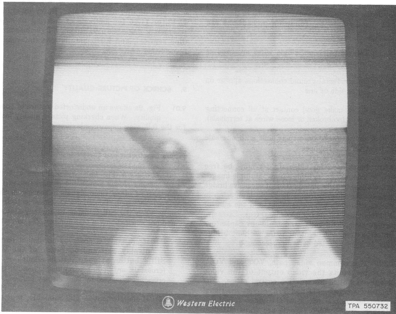
◆ Fig. 5—Image on Display Unit With One Side of Line (VIT or VIR) Open ◆
