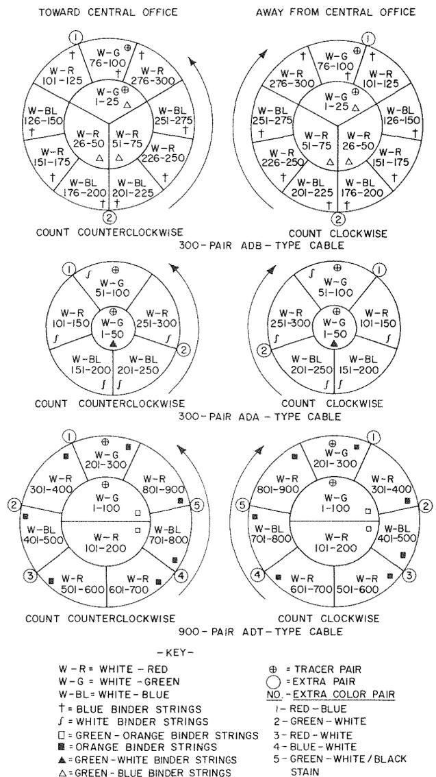
**Fig. 4 — Cable Count — Typical Straight Splices**
