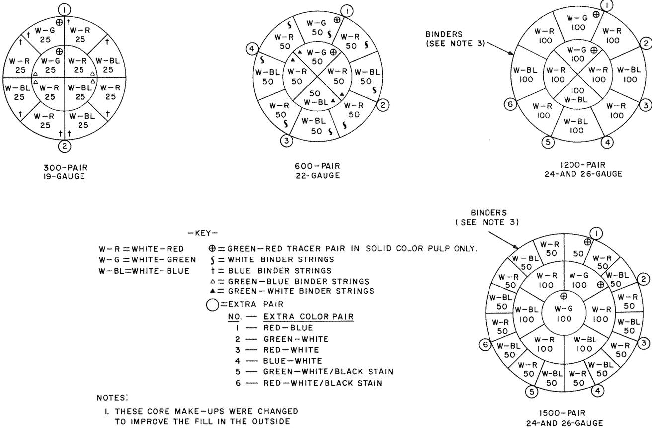
**Fig. 5 — Superseded Core Lay-Ups**
