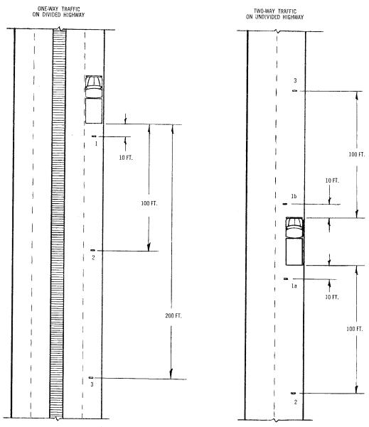
NOTE: Either position 1a or 1b may be used depending on which is better, considering road bends, vehicle position, etc.
