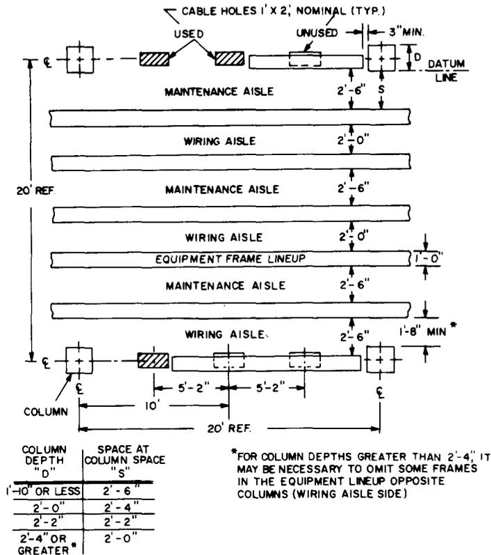
Fig. 3—Standard Floor Plan For Principal Dept (12 Inches) Frame
