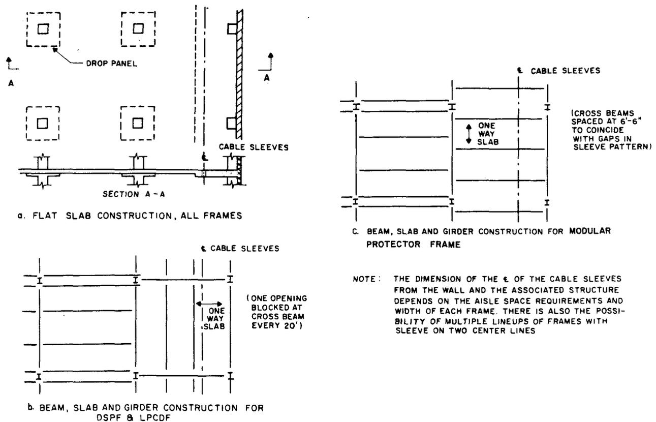
Fig. 5—Framing for Cable Holes Below Main Frames
