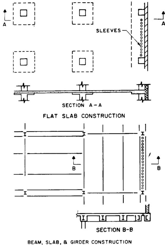
Fig. 6—Construction of Riser Openings
