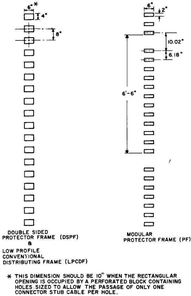
Fig. 4—Cable Hole Patterns for Various Frames
