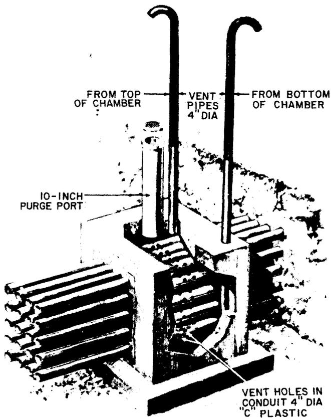
Fig. 2—Gas Venting Chamber (Trap) for Office With Above-Surface CEF
