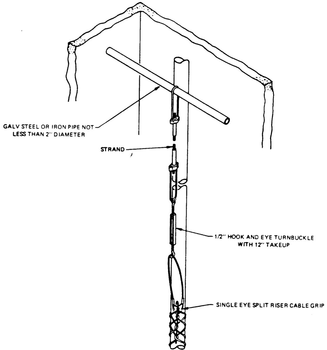
Fig. 10—Intermediate Cable Grip Support
