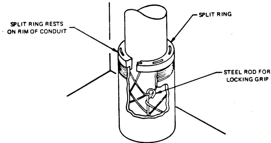
Fig. 9—Kellems Cable Grip With Split Ring Support (Fire Stop Not Shown for Clarity)
