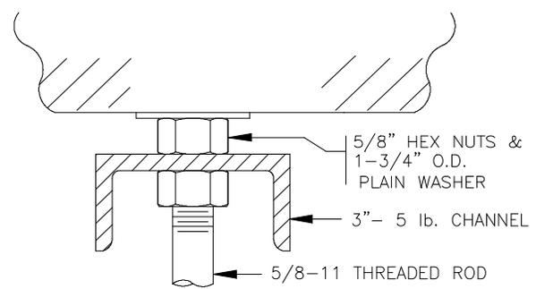
Fig. 12 - Hanger Rod Attachment At Ceiling
