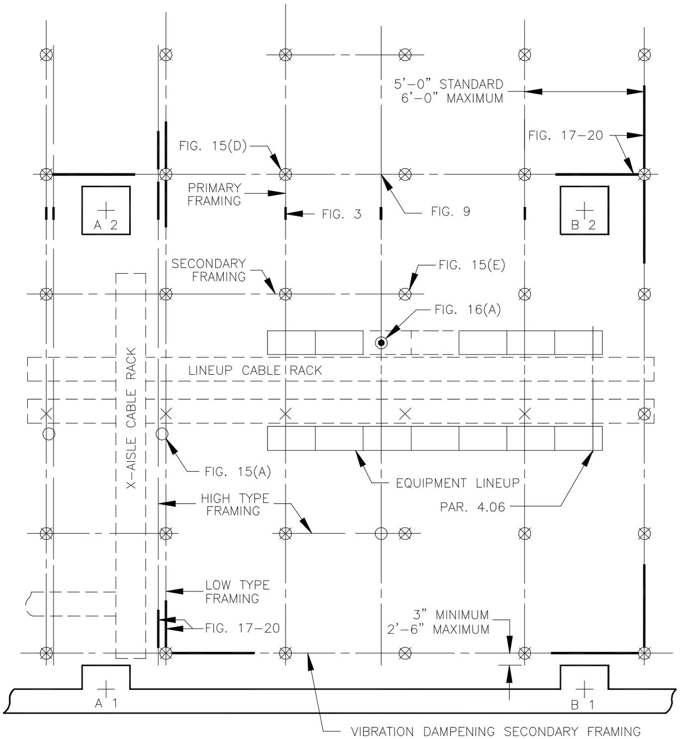
Fig. 1 - Typical Auxiliary Framing Arrangement Low Seismic Risk Areas
