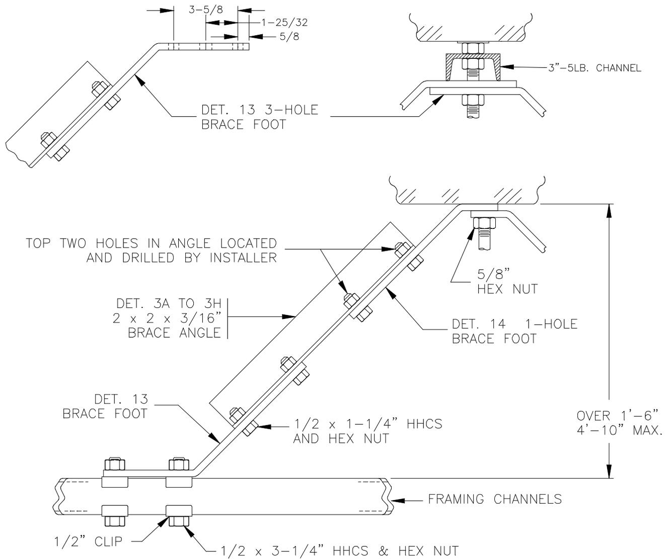
Fig. 20 - General Assembly Of Angle Type Braces
