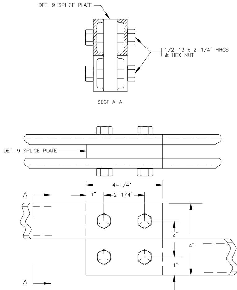
Fig. 6 - Splicing Of Auxiliary Framing Channels - 2 Inch Difference In Levels Of Channels
