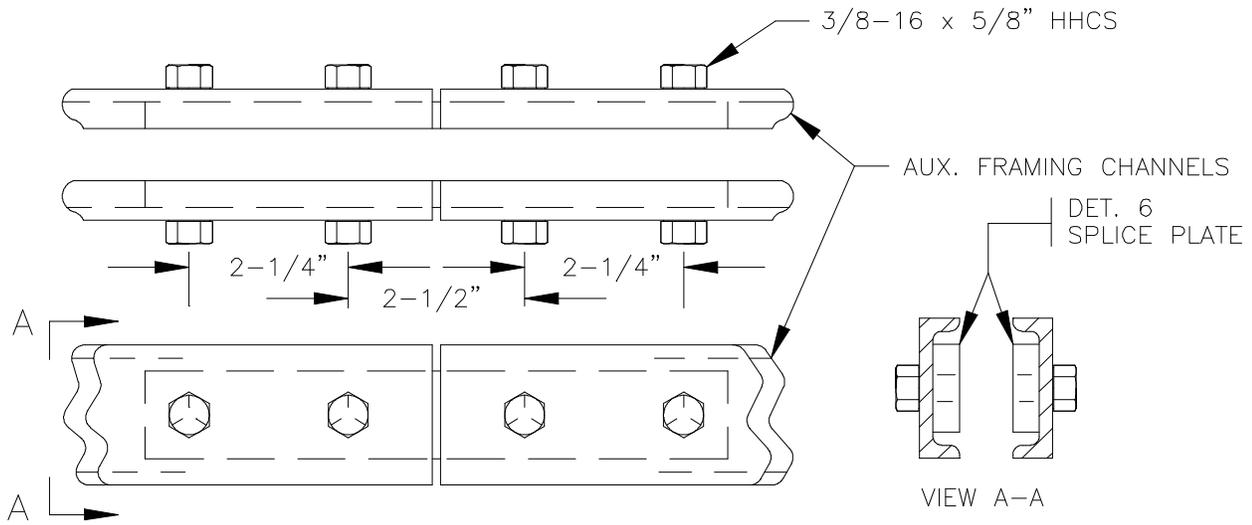
Fig. 3 - Splicing Of Auxiliary Framing
