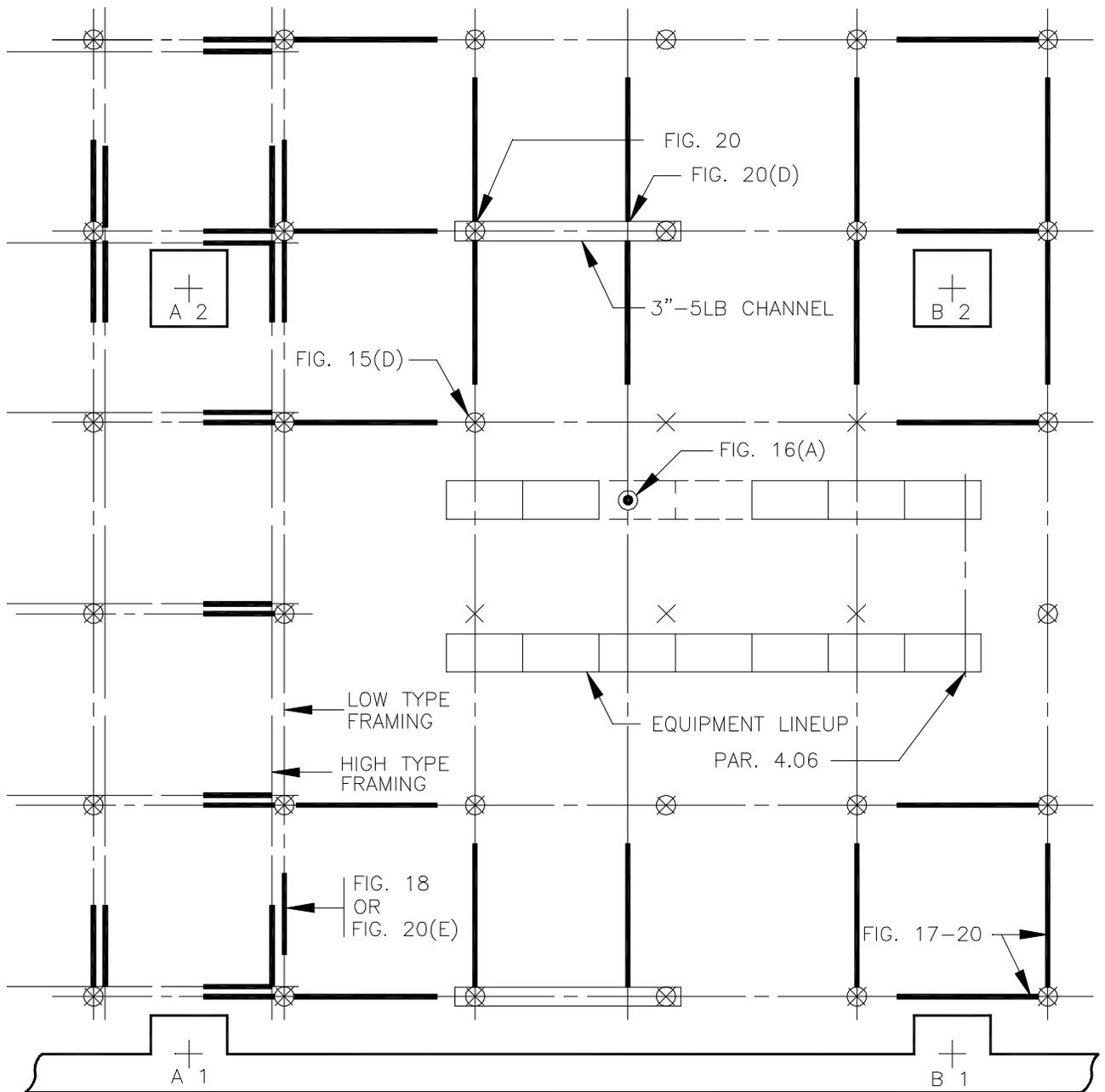
Fig. 2 - Typical Auxiliary Framing Arrangement High Seismic Risk Areas
