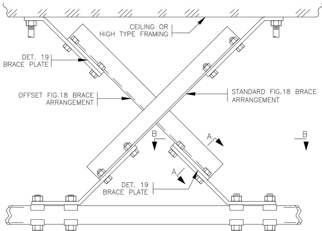
Fig. 27 - Method Of Installing Auxiliary Framing Braces At Same Location
