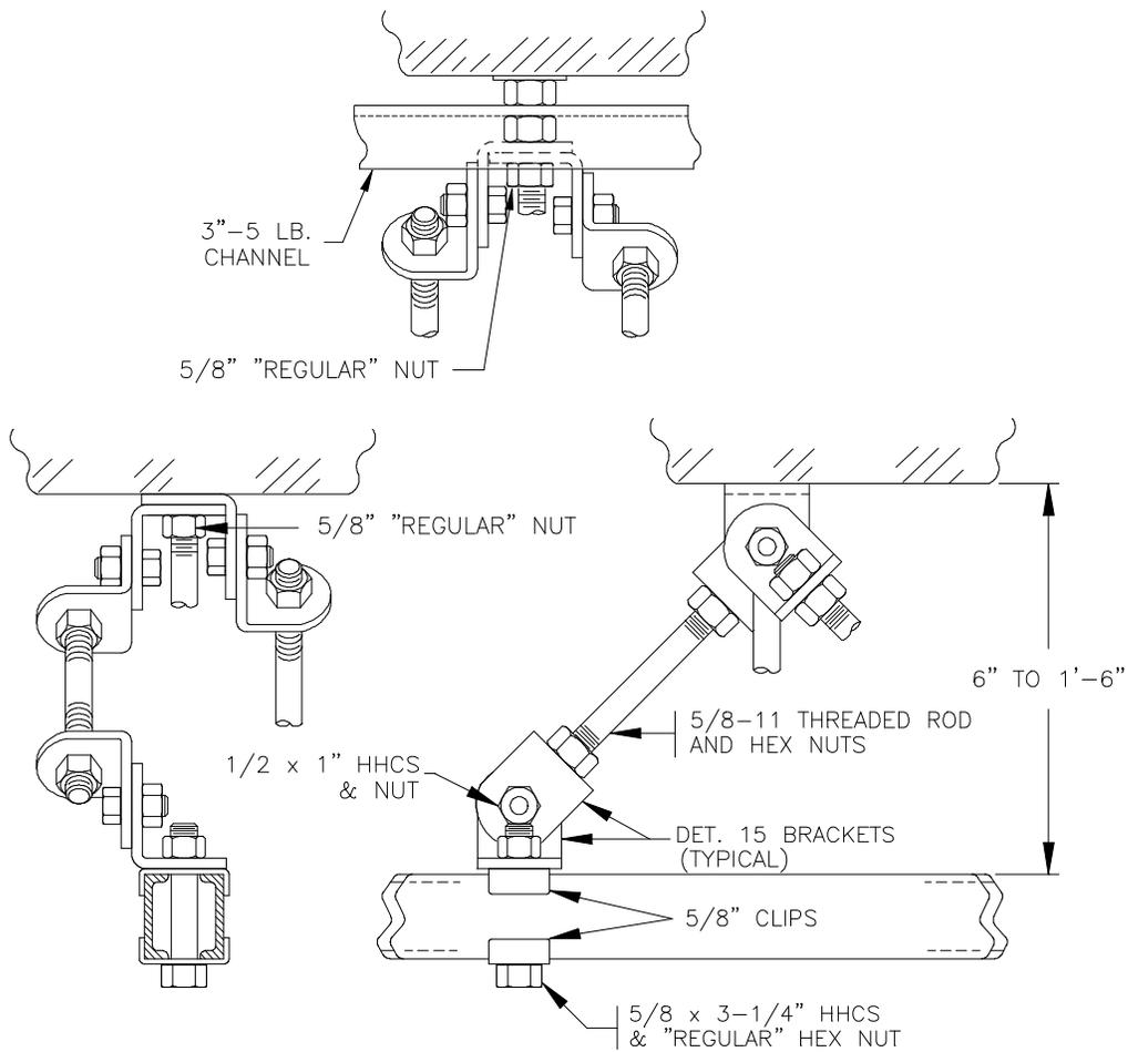
Single Or Double Rod From Support Rod/Ceiling Insert
