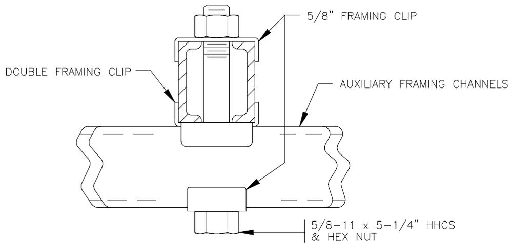
Fig. 9 - Auxiliary Framing Intersection - Double Level
