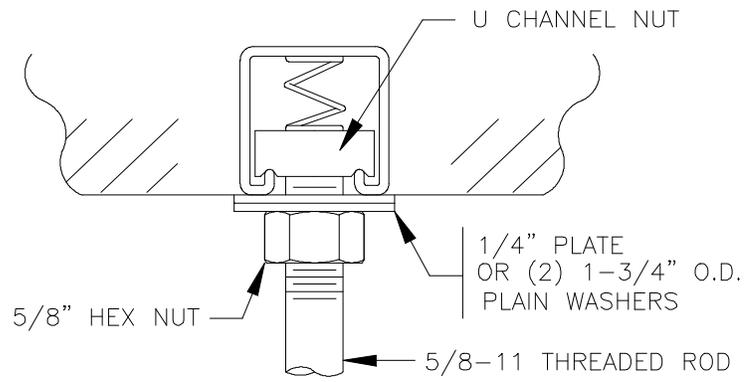
Fig. 13 - Hanger Rod Attachment At Ceiling Channel (Embedded Shown)
