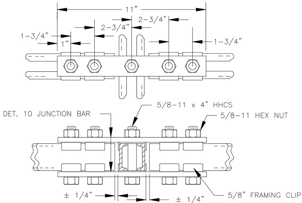
Fig. 7 - Auxiliary Framing Intersection - Single Level
