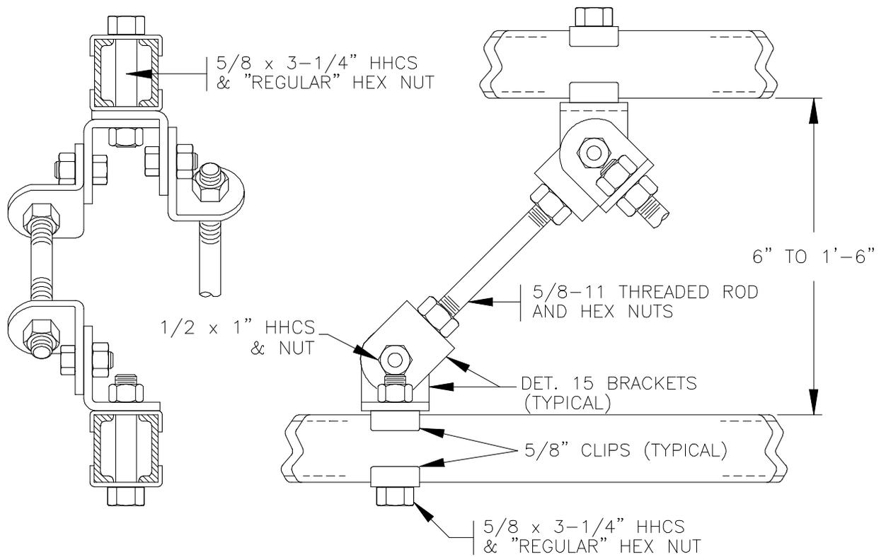
Fig. 18 - Threaded Rod Brace From Auxiliary Framing
