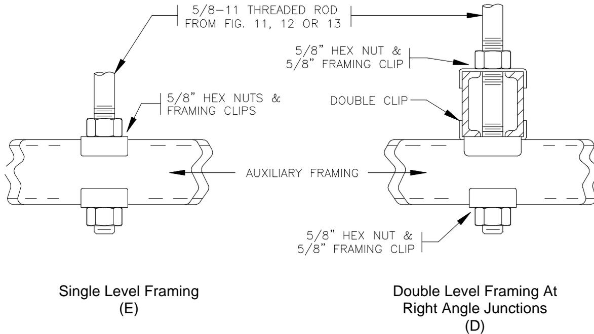
Fig. 15 - Support Of Auxiliary Framing From Ceiling Or Other Channels
