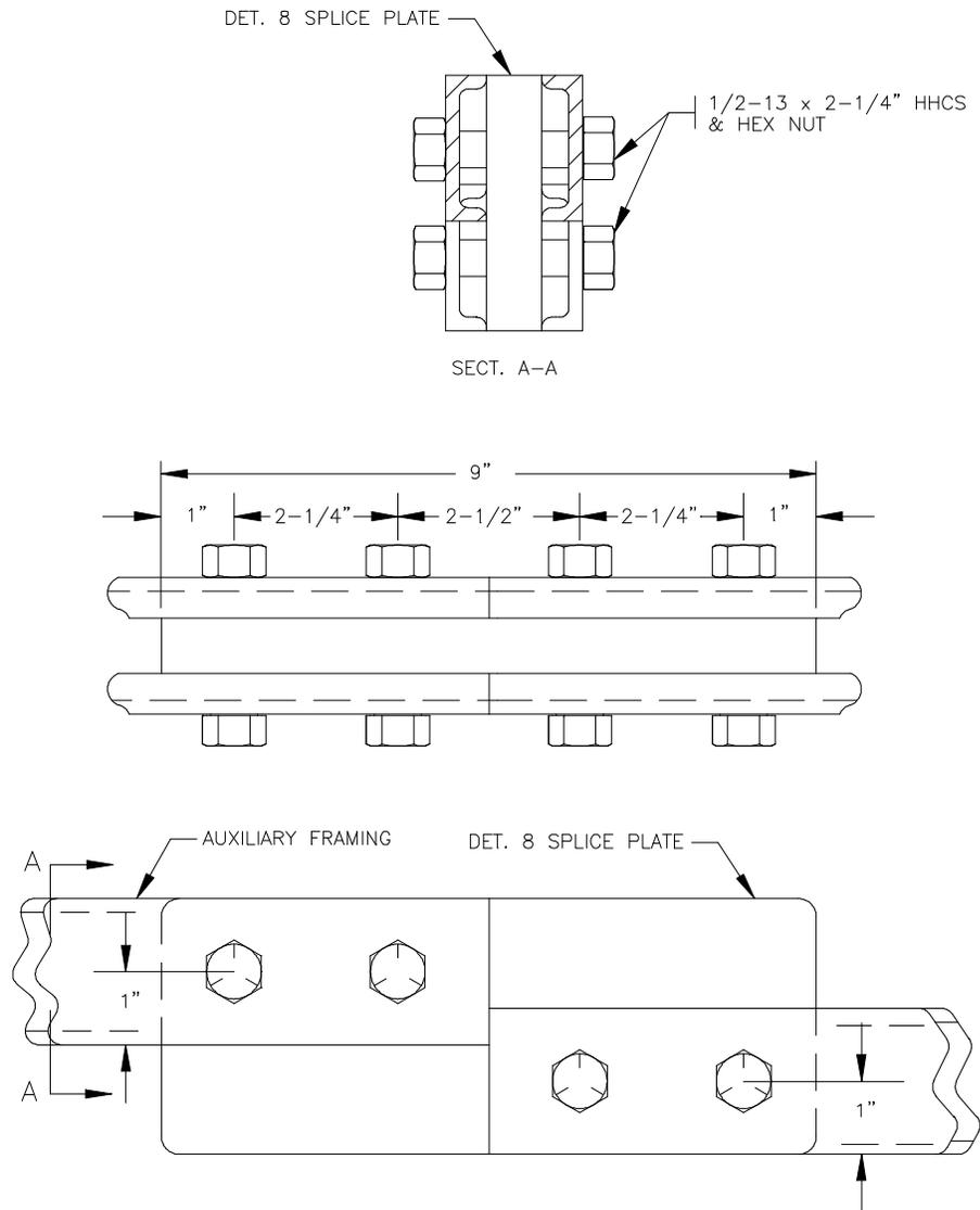
Fig. 5 - Splicing Of Auxiliary Framing Channels - 1-1/2 Inch Difference In Levels Of Channels
