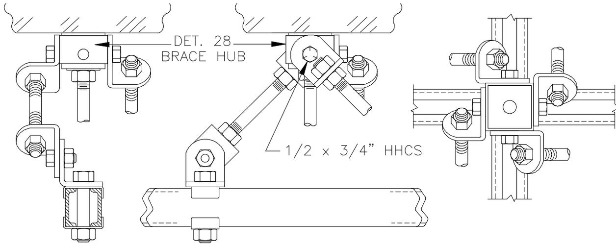
Three Or Four Braces From Support Rod/Ceiling Insert
