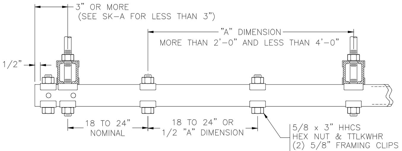
Fig. 25 - Arrangement Of Auxiliary Framing Stiffening Clips and Through-Bolts
