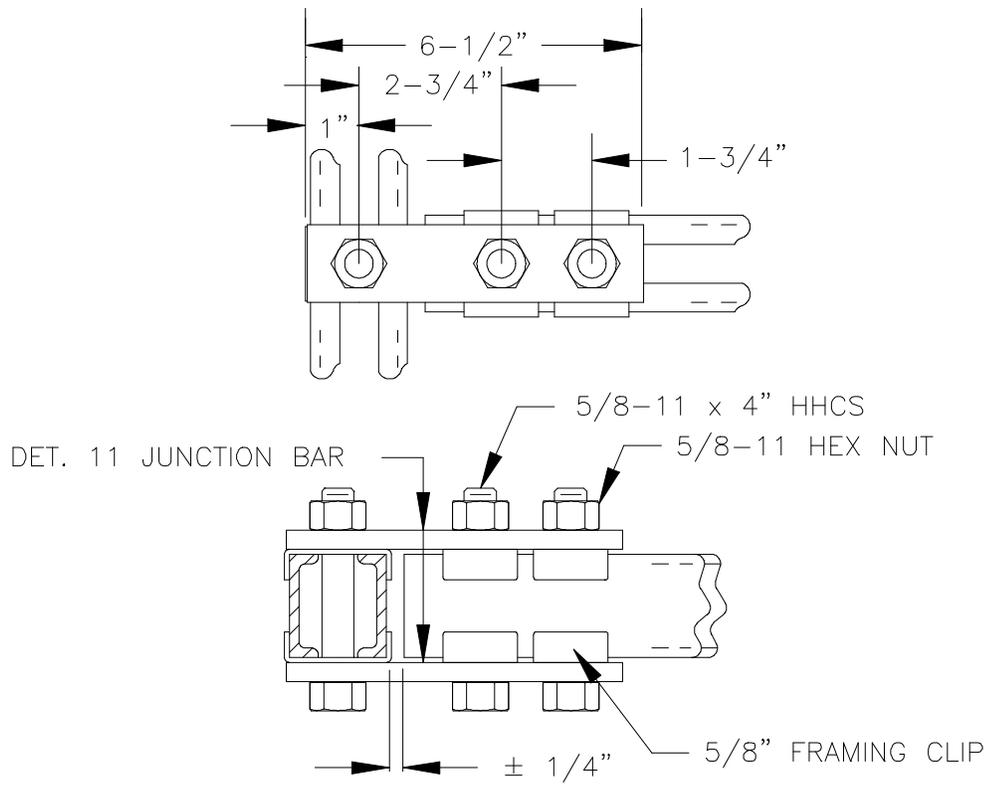
Fig. 8 - Auxiliary Framing Junction - Single Level
