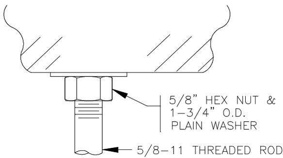
Fig. 11 - Hanger Rod Attachment At Ceiling
