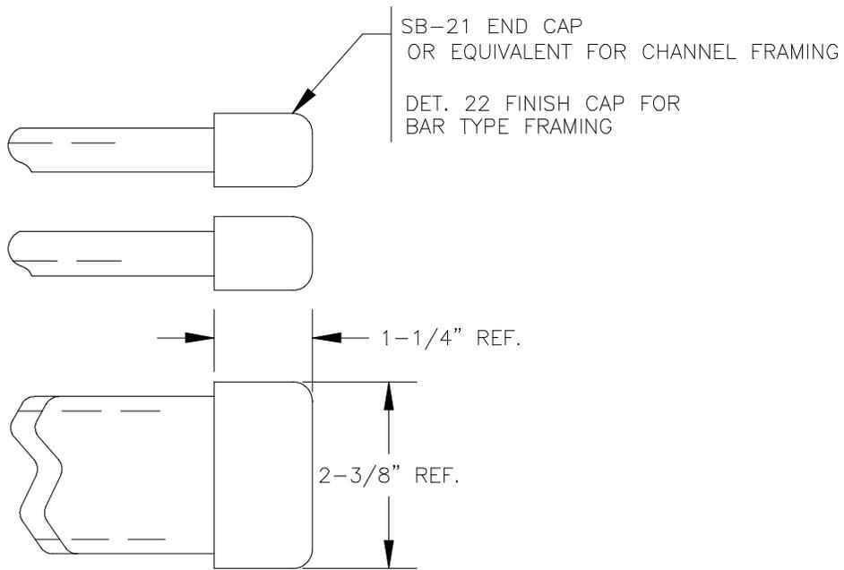
Fig. 10 - Auxiliary Framing Finishing Caps
