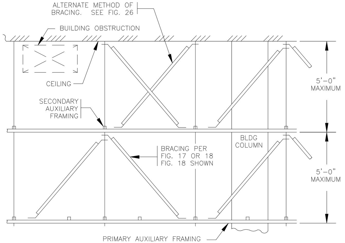
Fig. 26 - Typical Warren Truss Type Bracing Arrangement For Floor Supported Equipment Systems That Require Direct Attachment To Office Superstructure Via Framework Braces
