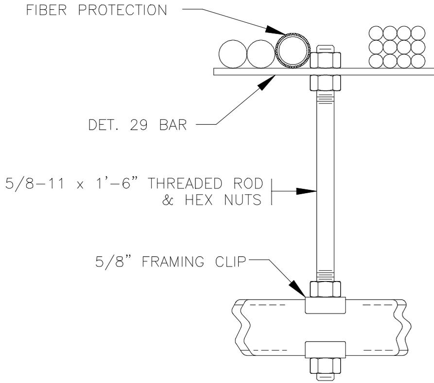
Fig. 29 - Auxiliary Cable Supports From Auxiliary Framing
