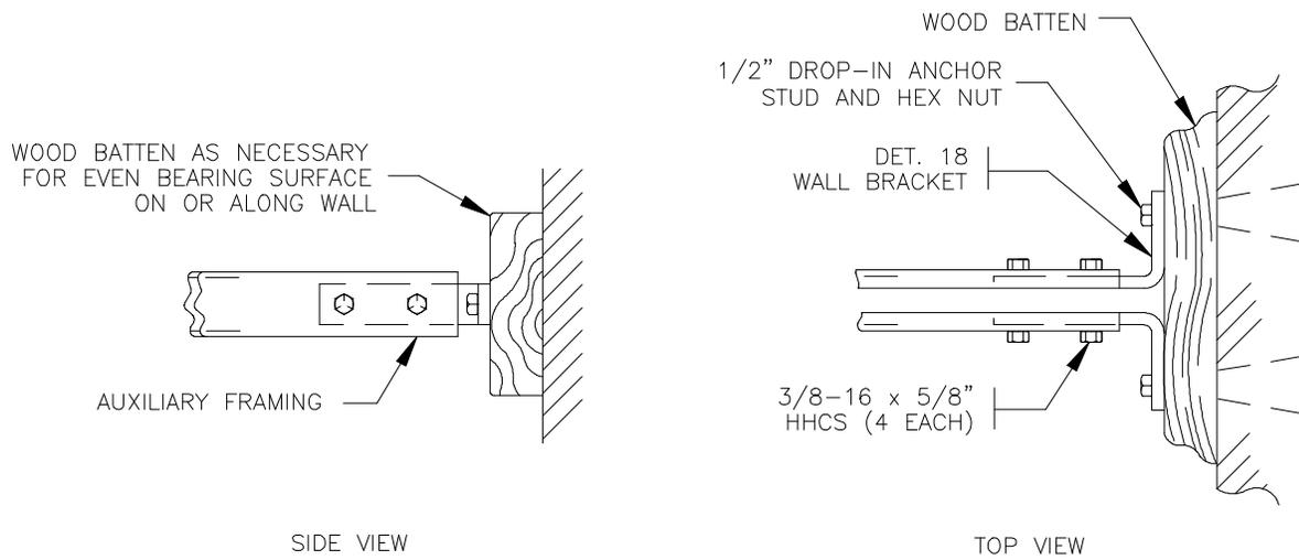
Fig. 23 - Auxiliary Framing Brace At Load Bearing Building Surfaces - High seismic risk areas
