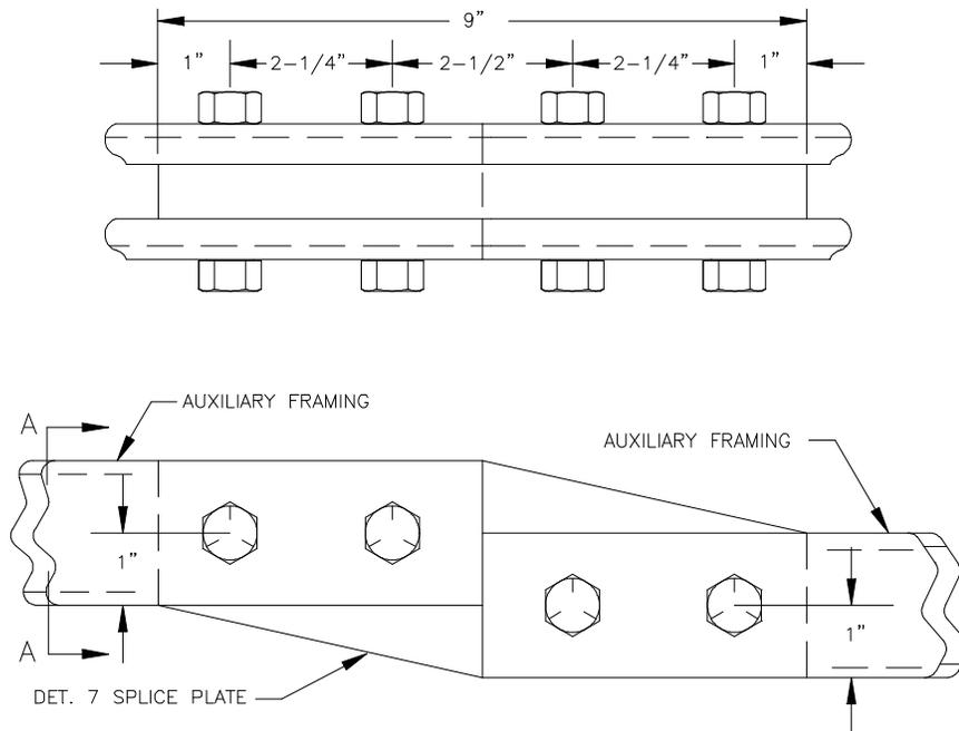
Fig. 4 - Splicing Of Auxiliary Framing Channels - 1 Inch Difference In Levels Of Channels
