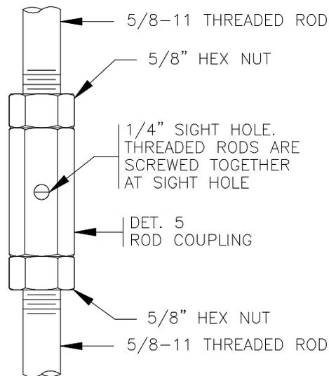
Fig. 14 - Hanger Rod Splice
