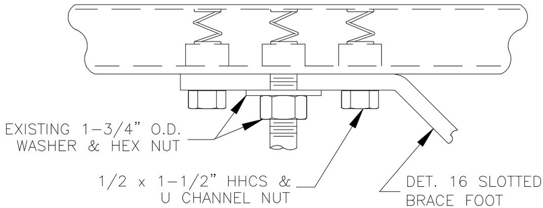
New Brace To Existing Rod At Ceiling Channel Installed Parallel To Auxiliary Framing (B)
