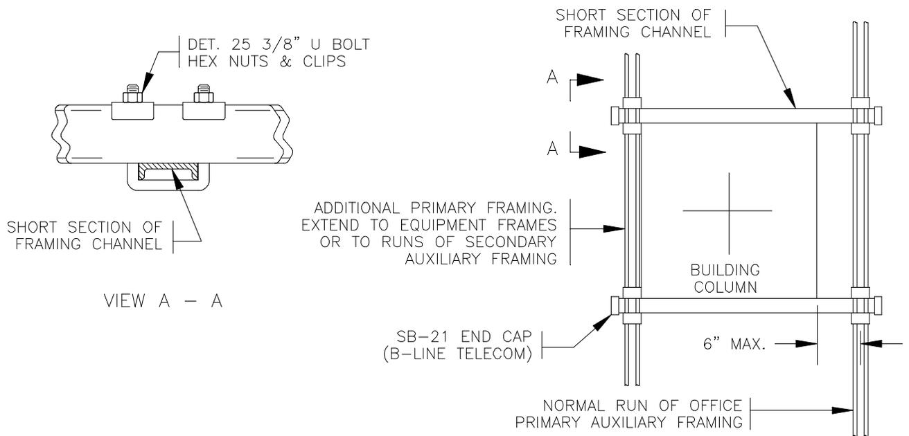
Fig. 24 - Auxiliary Framing Brace At Building Column
