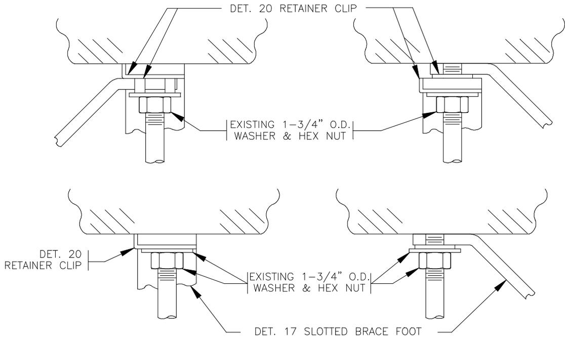
New Brace To Existing Rod At Ceiling Insert Or Ceiling Channel Installed At A Right Angle To Auxiliary Framing (A)
