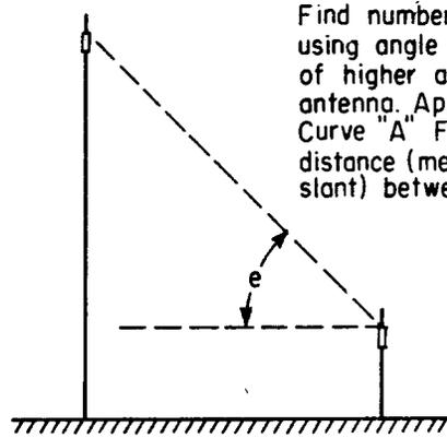
Find number of db additional using angle of elevation  $e$  of higher antenna from lower antenna. Apply correction to Curve "A" Fig. 6 using actual distance (measured along slant) between antennas.
