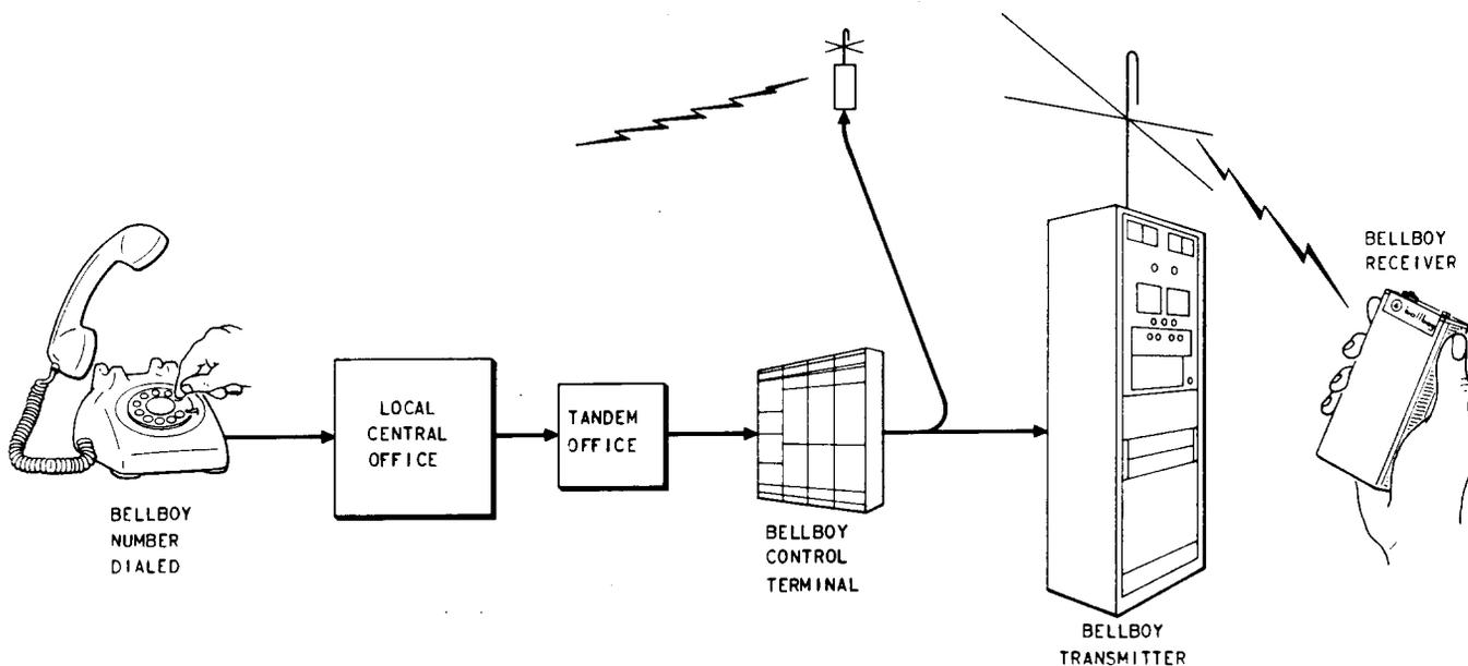
Fig. 1—Typical Setup for a BELLBOY Call
