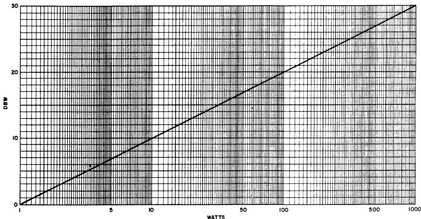
Fig. 7—Power in dBW vs Watts
