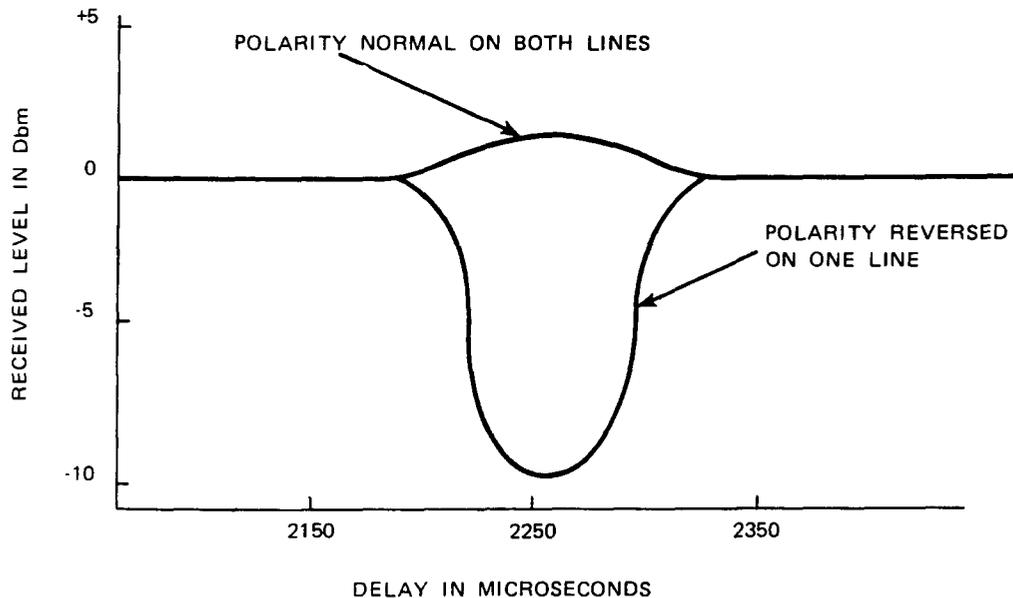
**Fig. A.1—Polarity Effect Using 1000-Hz Tone**
