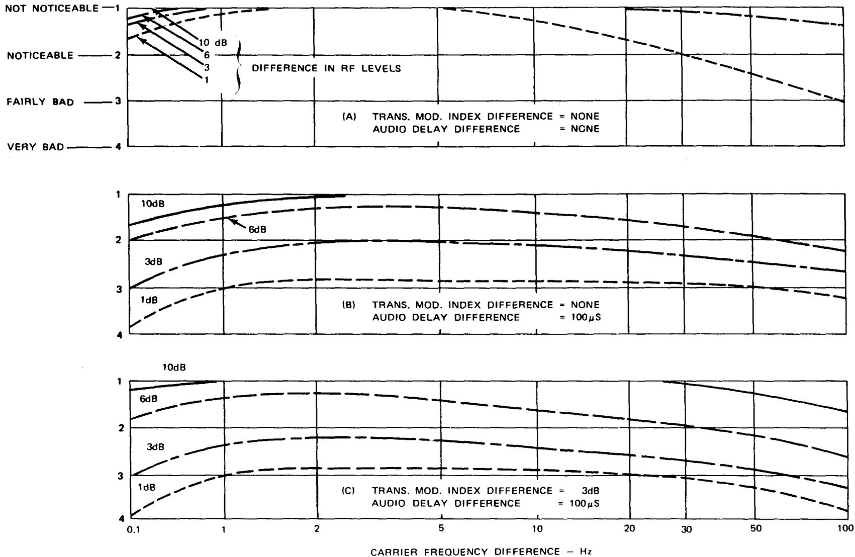
Fig. 1—Subjective Evaluation of Speech Degradation Resulting From Presence of Two Signals at Receiver Input
