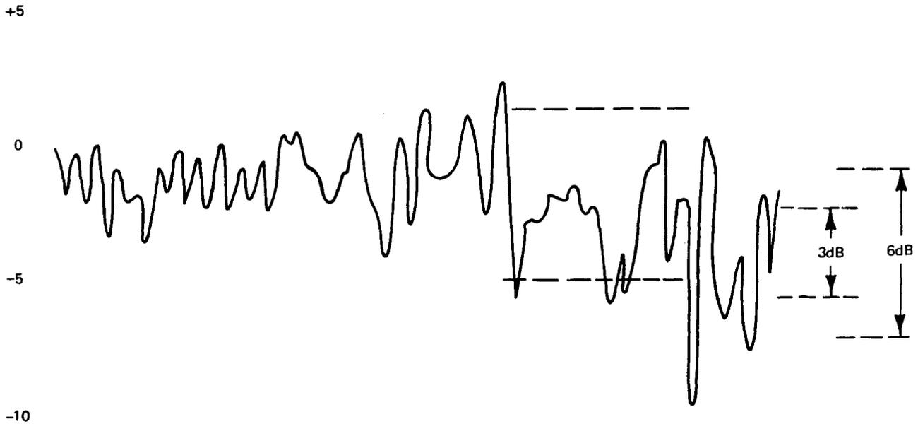
Fig. 2—Variation of 152-MHz Signal Level Along Street in Relatively Level Area
