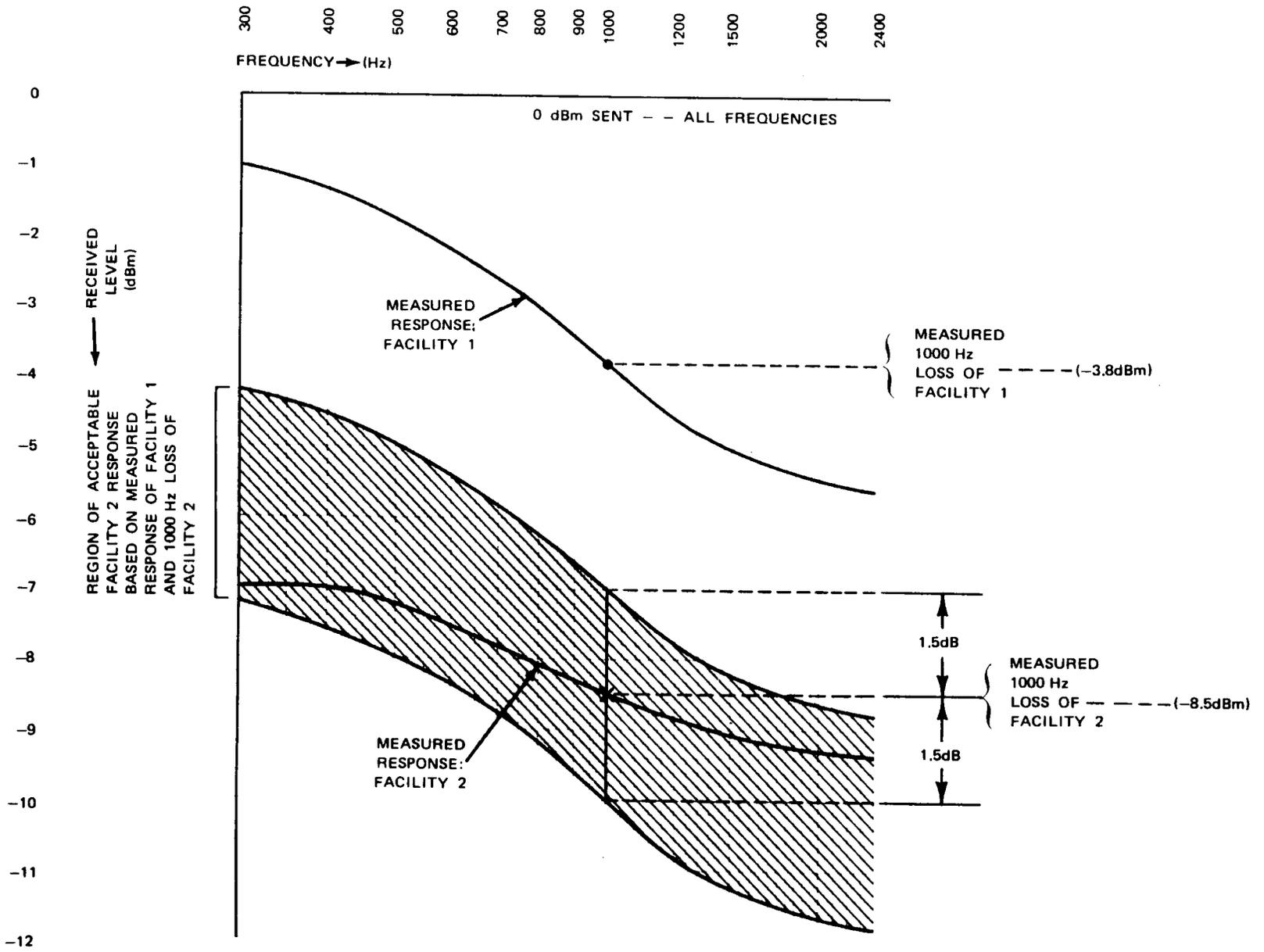
Fig. 3—Measured Amplitude Response of Equalized Transmitter Land-Line Facilities
