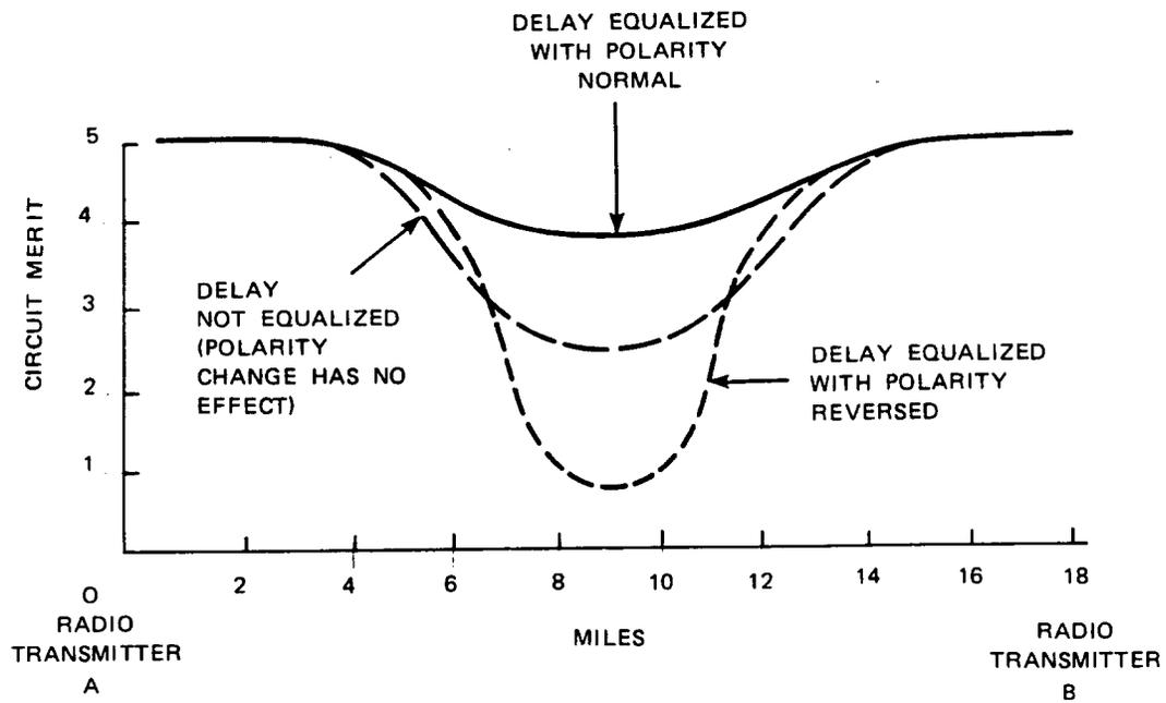
Fig. A.2—Effect of Polarity on Voice Transmission
