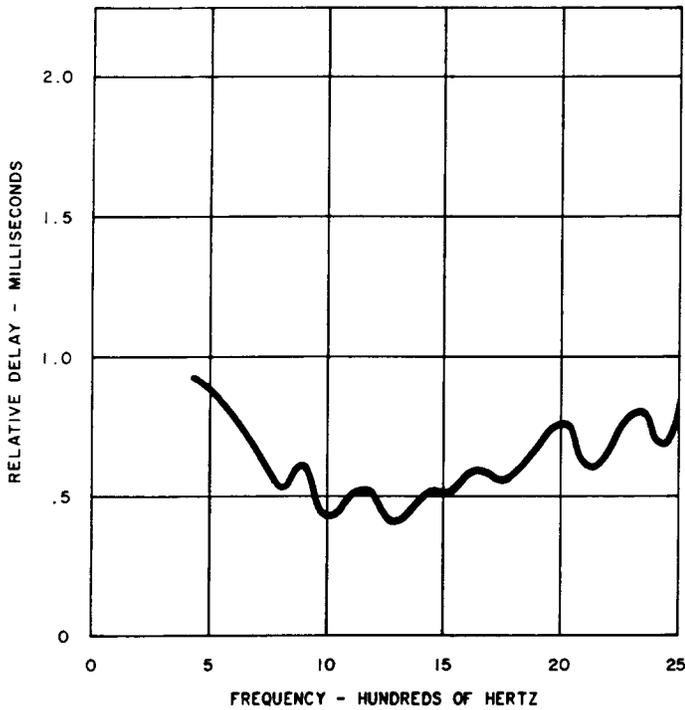
Fig. 4—Circuit Layout Record of Envelope Delay
