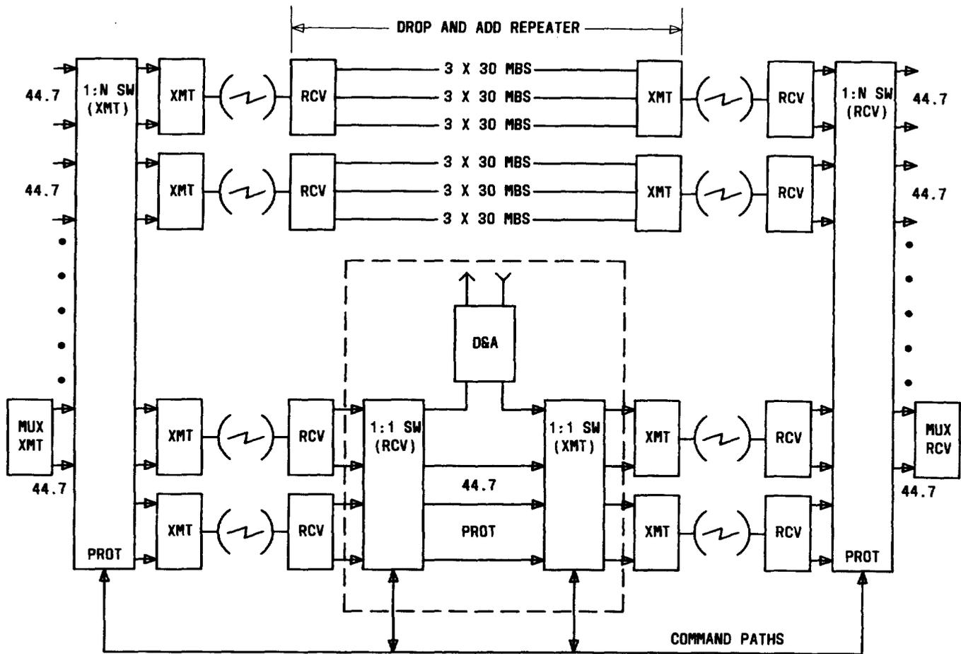
Fig. 8—1:N With Drop and Add Repeater (90-Mb System Shown)
