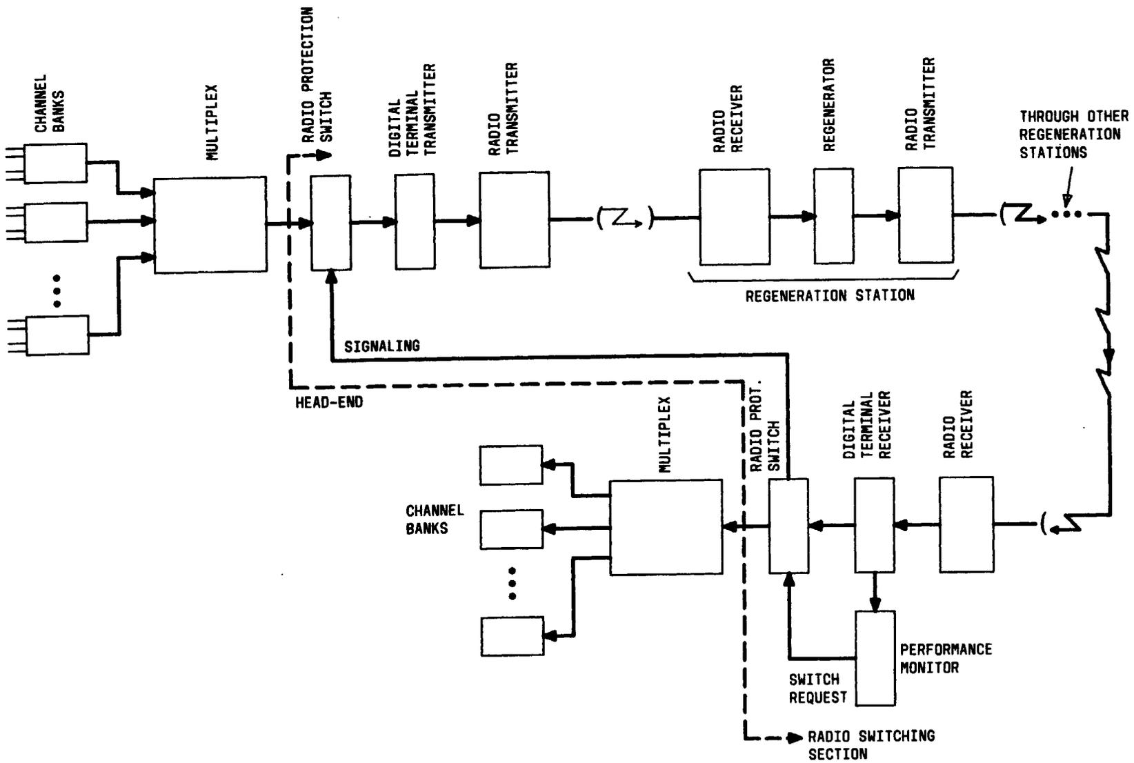
Fig. 7—Radio Switching Section—Block Diagram
