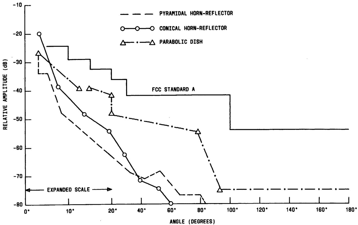
Fig. 13—Antenna Radiation Patterns (Horizontal Polarization, 6 GHz)
