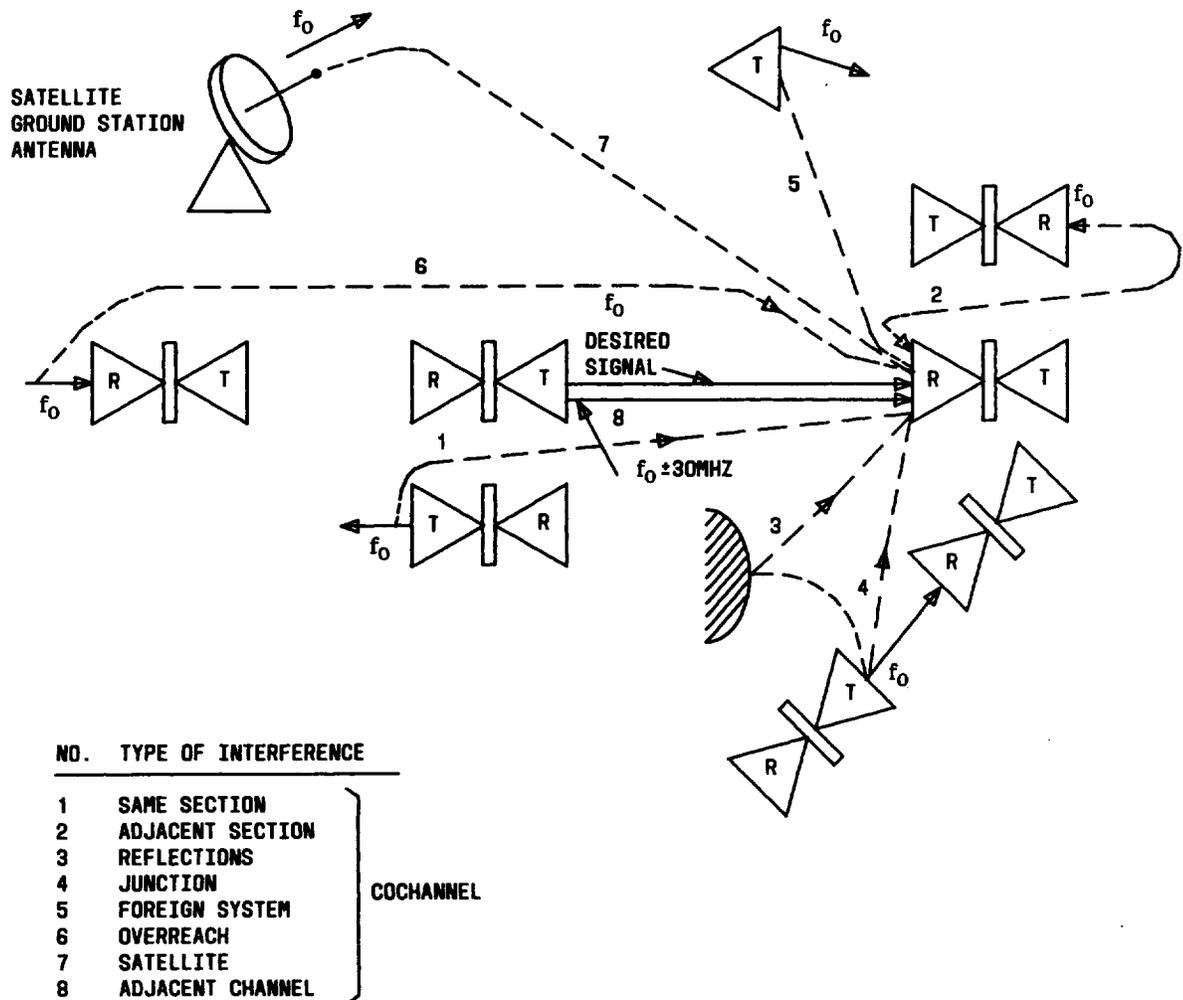
Fig. 11—Sources of Interference (6 GHz)
