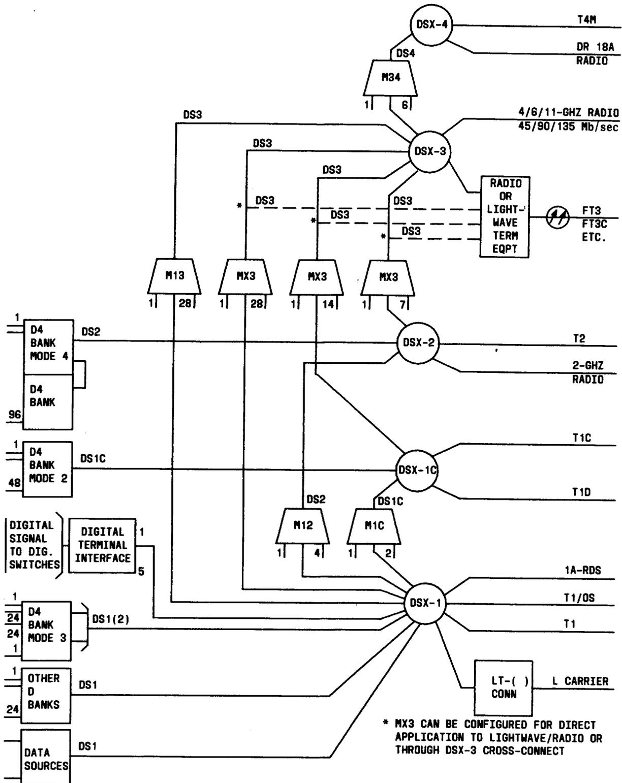
Fig. 1—Digital Hierarchy and Transmission Facilities
