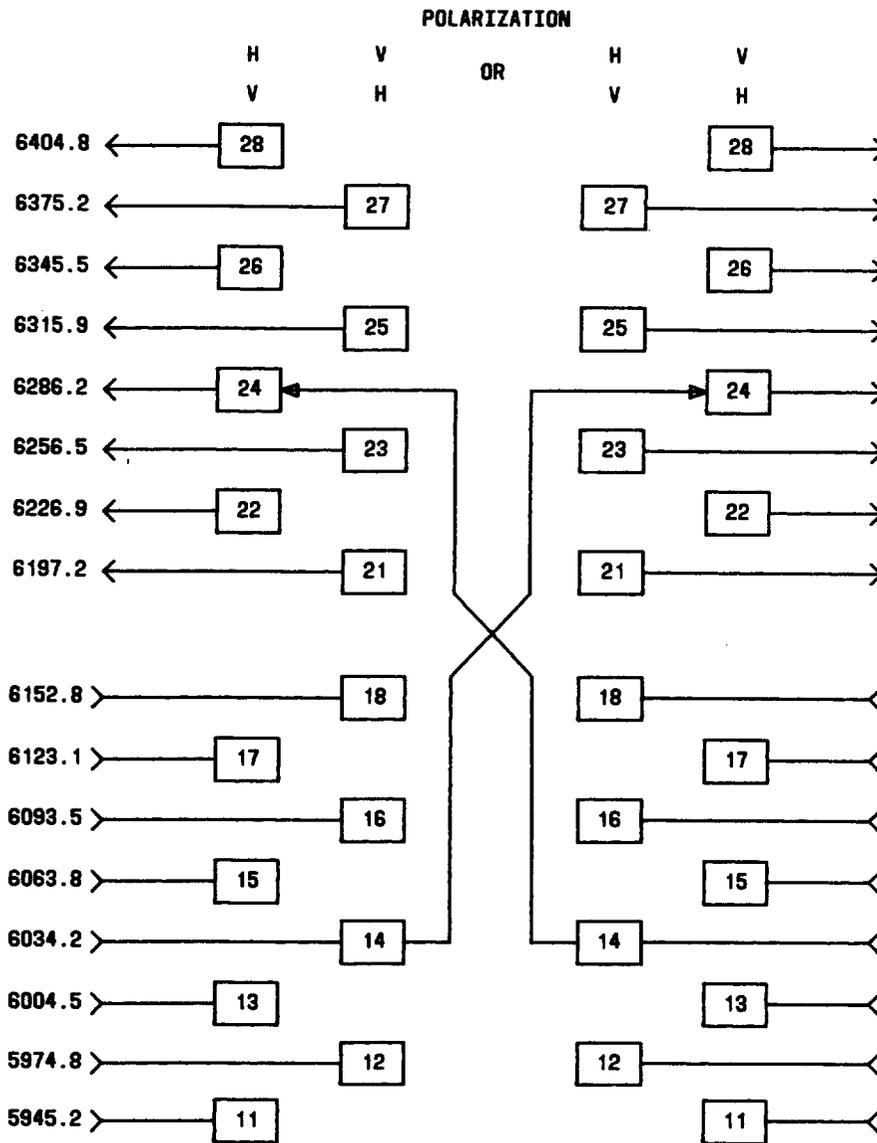
Fig. 3—Frequency Plan
