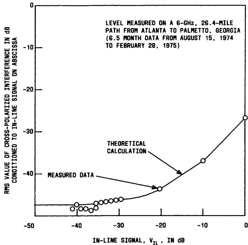
Fig. 12—Dependence of RMS Value of Cochannel Cross-Polarization Interference on In-Line Signal Level
