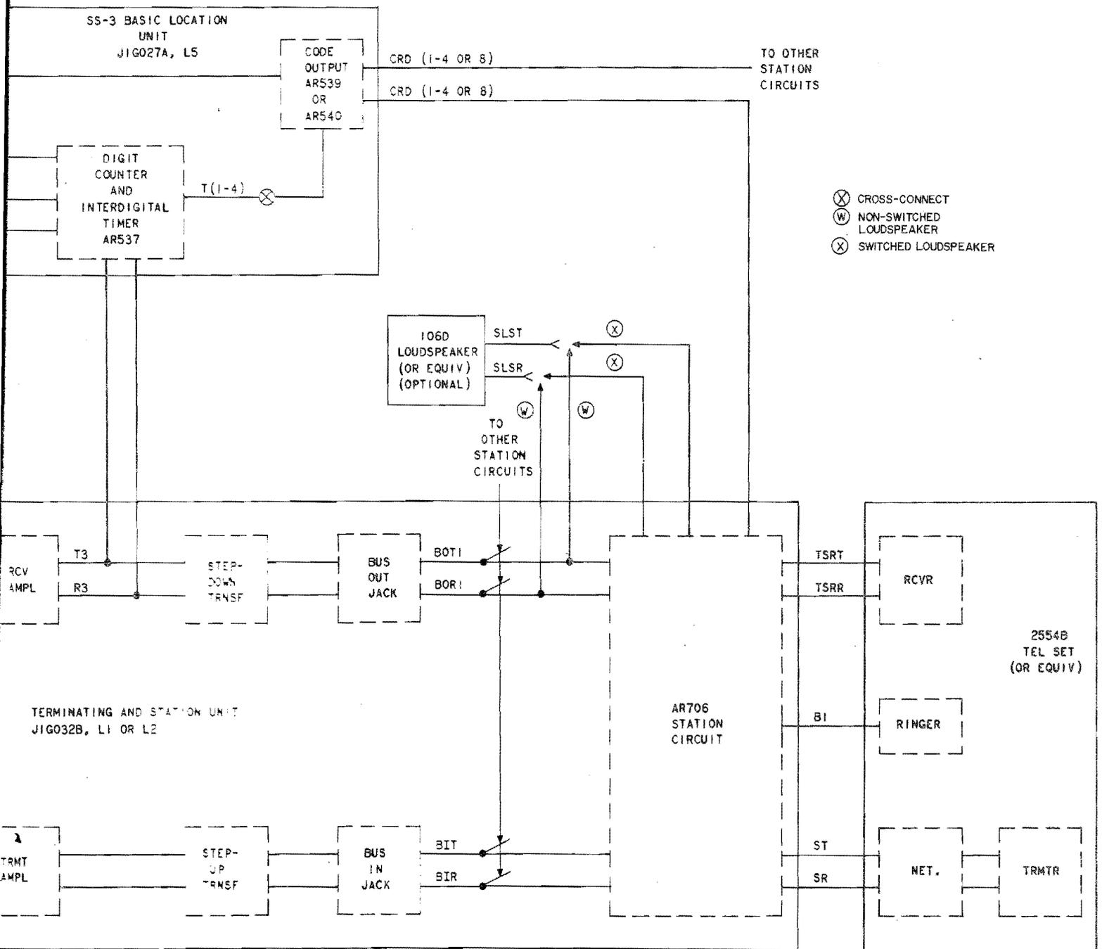
Fig. 4—Block Diagram of Single Line-Single Station Units
