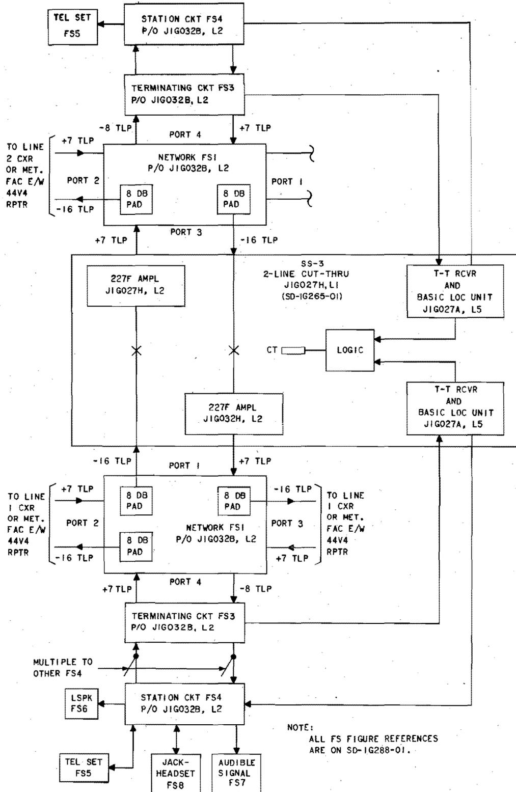
Fig. 10—2-Line Cut-Through Switch Installation—With Terminating and Station Equipment on Both Lines
