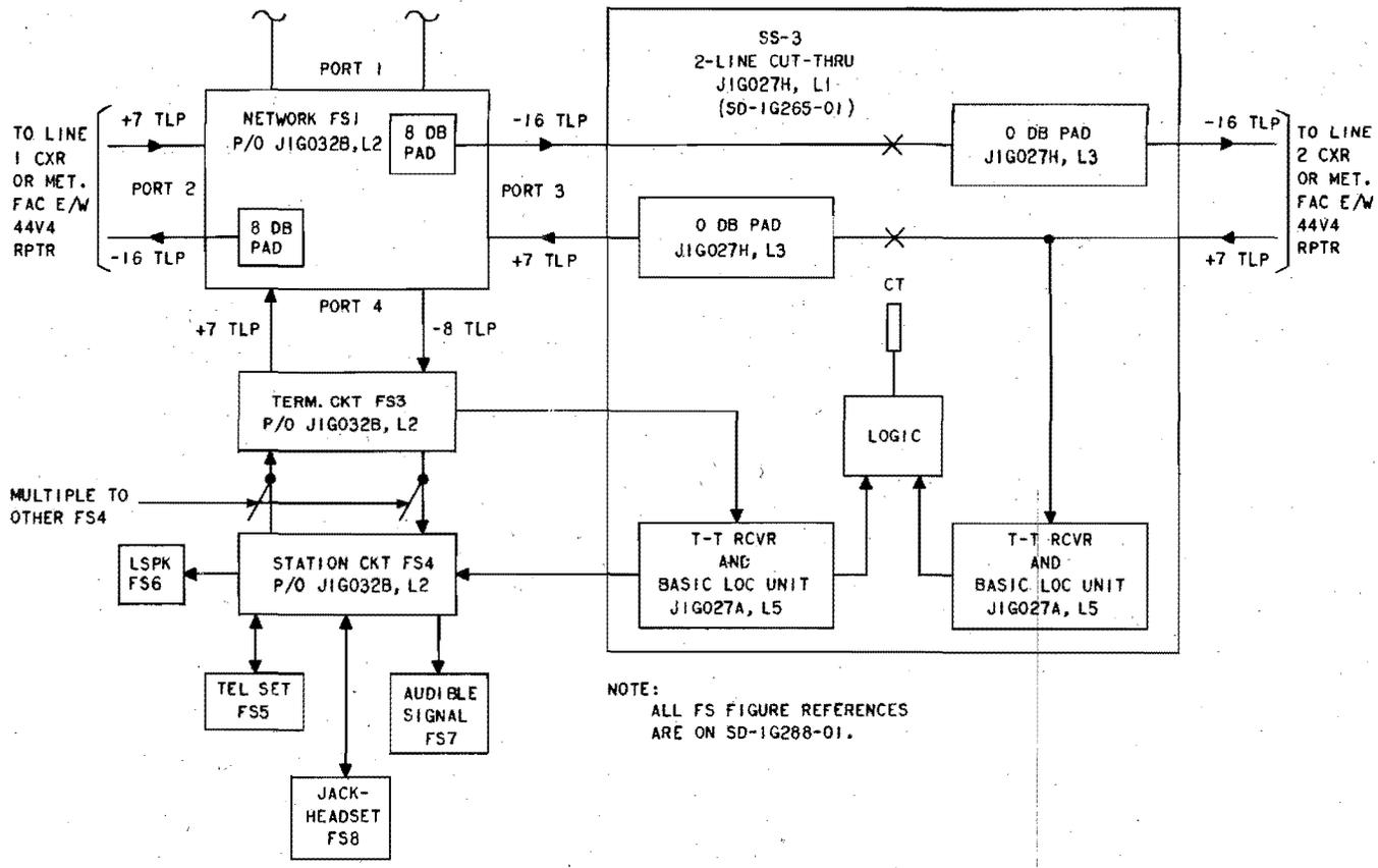
Fig. 9—2-Line Cut-Through Switch Installation—With Terminating and Station Equipment on One Line
