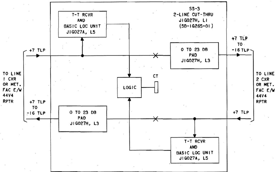
Fig. 8—2-Line Cut-Through Switch Installation—Without Terminating and Station Equipment
