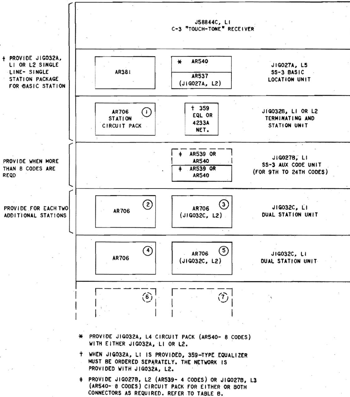
Fig. 5—Typical Equipment Arrangement for Multiple Station Installation
