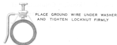
Fig. 14 — Terminating Sequence — Ground Clamp
