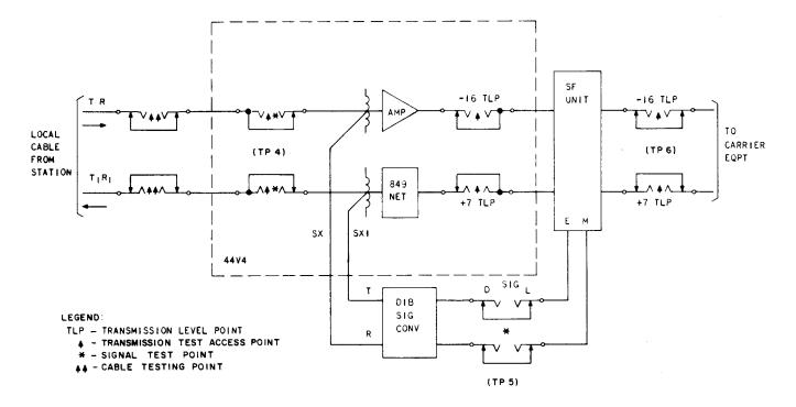
Fig. 3—Typical Central Office Arrangement for Two-Point Private Line Telephone Service and Test Access Points
