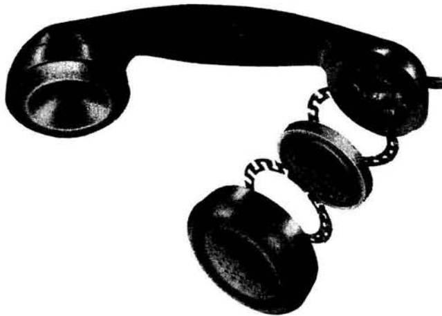
Fig. 20 — KS-14200 Lock, Order of Assembly
