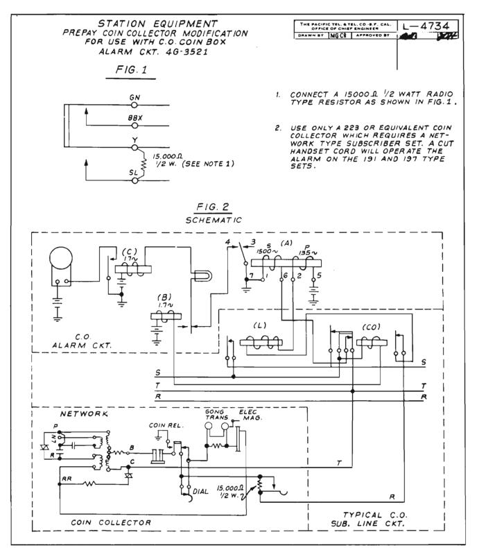
Fig. 1 - Schematic of coin station and line circuit modified for coin box alarm circuit 4G-3521.
