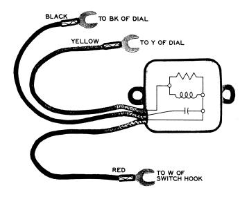
Fig. 6—61N Filter Connections
