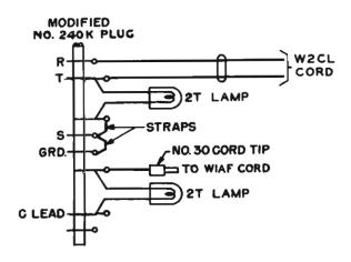
Fig. 2 - Modification at the No. 240K Plug
