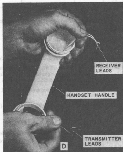
Fig. 11D—Handset Cord Replacement
