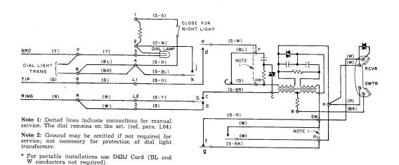
Fig. 1-701B Telephone Set without Ringer, or Portable
