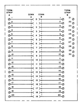
Fig. 3—259B KTU Schematic, Arrangement of Screw Terminals
