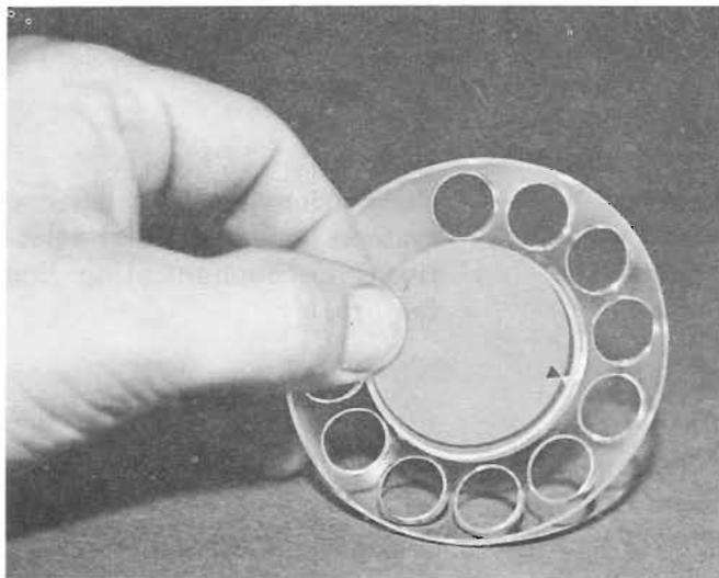
7.02 To install modified station number card in P-11E007 dome-type finger wheel, insert number card (do not remove perforated notch) with point of arrowhead, printed on back of card, touching triangular tip of molded lucite inside finger wheel (see Fig. 24). Next, insert card support, if required, into frame, making certain card support is seated firmly to ensure proper locking in frame.
