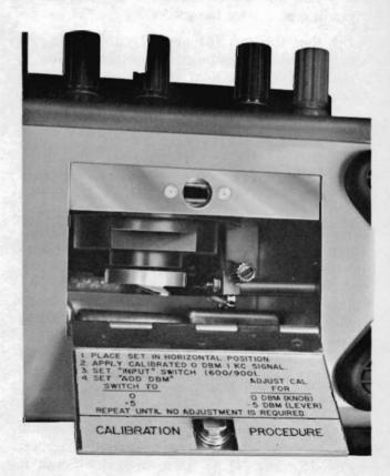
Fig. 5 - Calibration Controls
