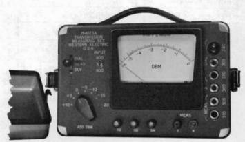
Fig. 1 - The 23A Transmission Measuring Set
