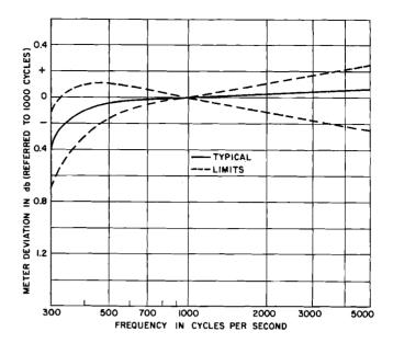
Fig. 4 – Frequency Characteristic of the 23A
