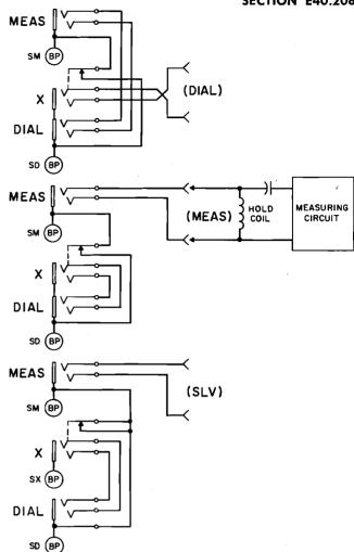
Fig. 3 - Schematic Circuit of the DIAL-MEAS-SLV Key
