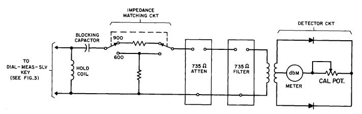
Fig. 2 - Simplified Schematic, 23A Transmission Measuring Set
