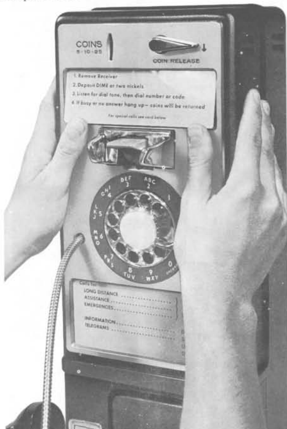
Fig. 12—Installing Instruction Card (Typical)
