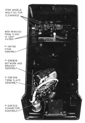
Fig. 2—Upper Housing With Gong Signal and Chute
