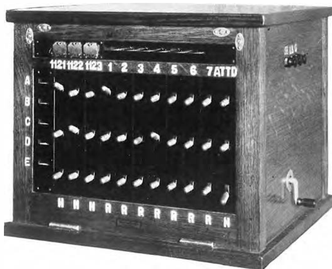
Figure 14 Extensions No. 1 and No. 4 Connected with Trunks for Night Service
