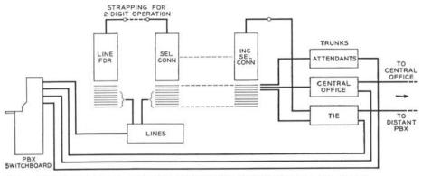
Fig. 1-Circuit arrangement of the 740-E where three-digit numbers are not required.
