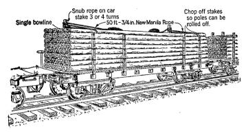
Stakes on the unloading side shall then be cut off to a level such that the poles in the top layer can be rolled past them.
