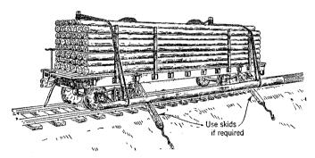
2.04 Before the train is started the skids shall be slung into the carrying position and the next pole to be unloaded shall be snubbed as previously described.
