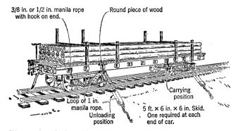
The ends of the skids which rest on the ground when in the unloading position should be toward the rear of the train when in the carrying position. 2.02 Upon reaching the destination at which unloading is commence the wire on the top of the load shall be removed. The pole in the uppermost layer on the side on which poles are to be unloaded shall be snubbed as shown below.
