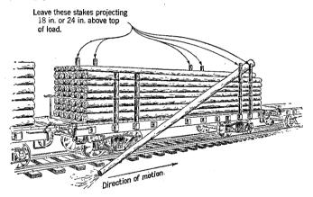
3.02 It will usually be necessary to secure the first pole in each layer by means of a rope sling about the end toward the rear of the car, as the stakes at this end of the car are chopped off. This will prevent poles from accidentally rolling off the load. Poles can be secured as illustrated in para-
