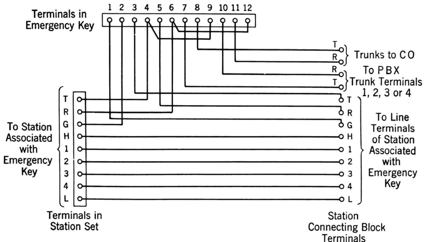
**Fig. 18 – Emergency Trunk Key Wiring**
