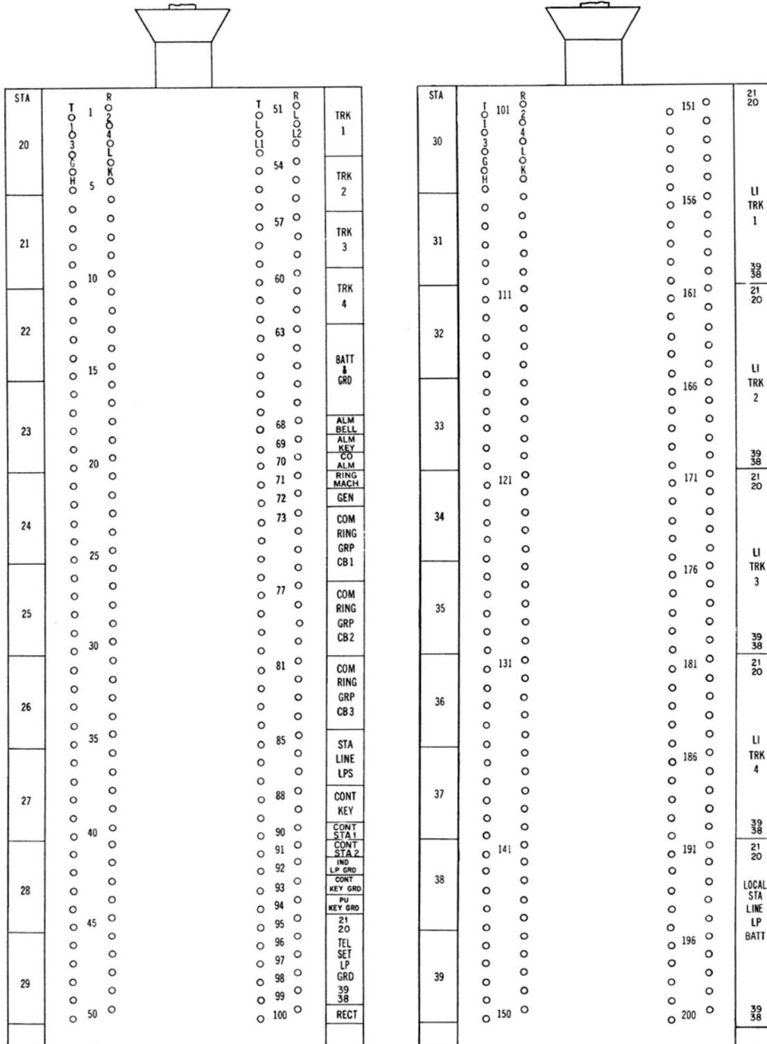
For a 20 line installation use 2-100 pair binding post chambers.
