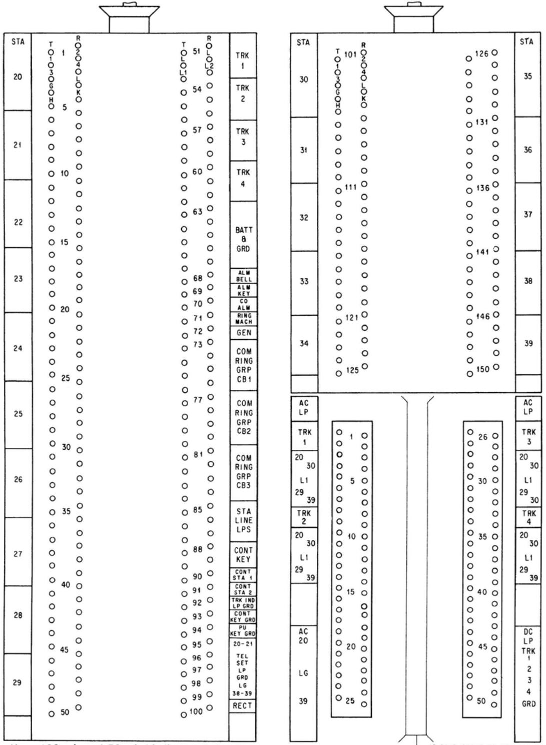
Use a 100pair and 50pair binding post chamber, appropriate type conn blocks, and fanning strips. Terminate station lines as shown for stations 20 to 29. Pair numbers not to be stamped.
