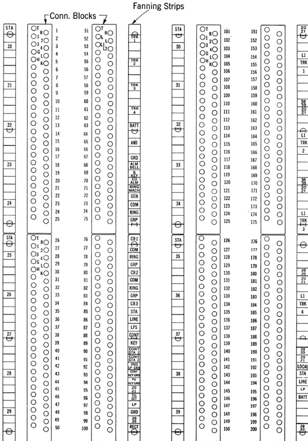
Use Cables of proper size to give 200 pairs to P.B.X term. strips A and B. Pair numbers not to be stamped.
