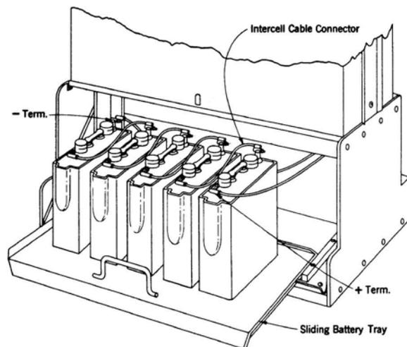
**Fig. 15 — Battery Connections**
