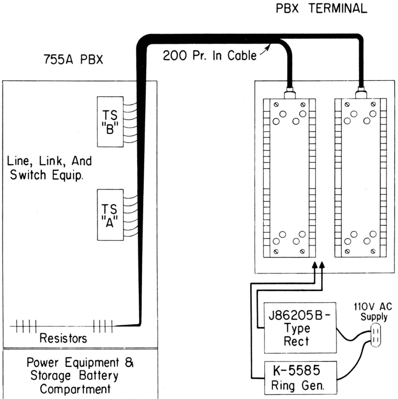
Fig. 2 — Typical Arrangement of 20-Line PBX — Lamp Power from PBX
