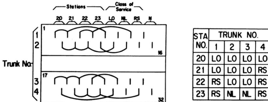
Fig. 17 – Connections at 224-Type CS (Class of Service) Terminal Strips
