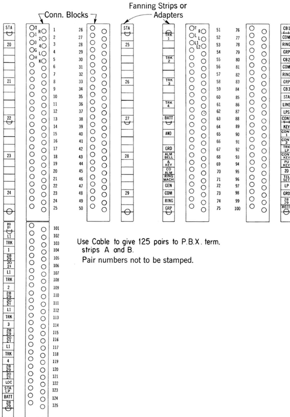
Fig. 5 — Arrangement of Connecting Blocks — 10-Line Size — Lamp Power from PBX
