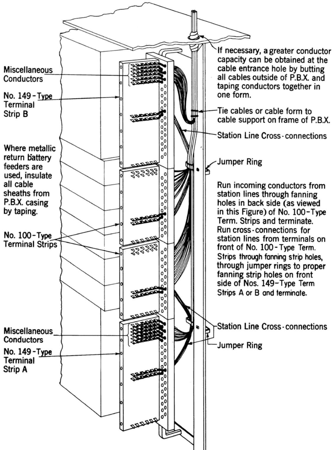
**Fig. 12 — Typical Cabling of PBX Where Cross Connections are Made at the PBX Terminal Strips**
