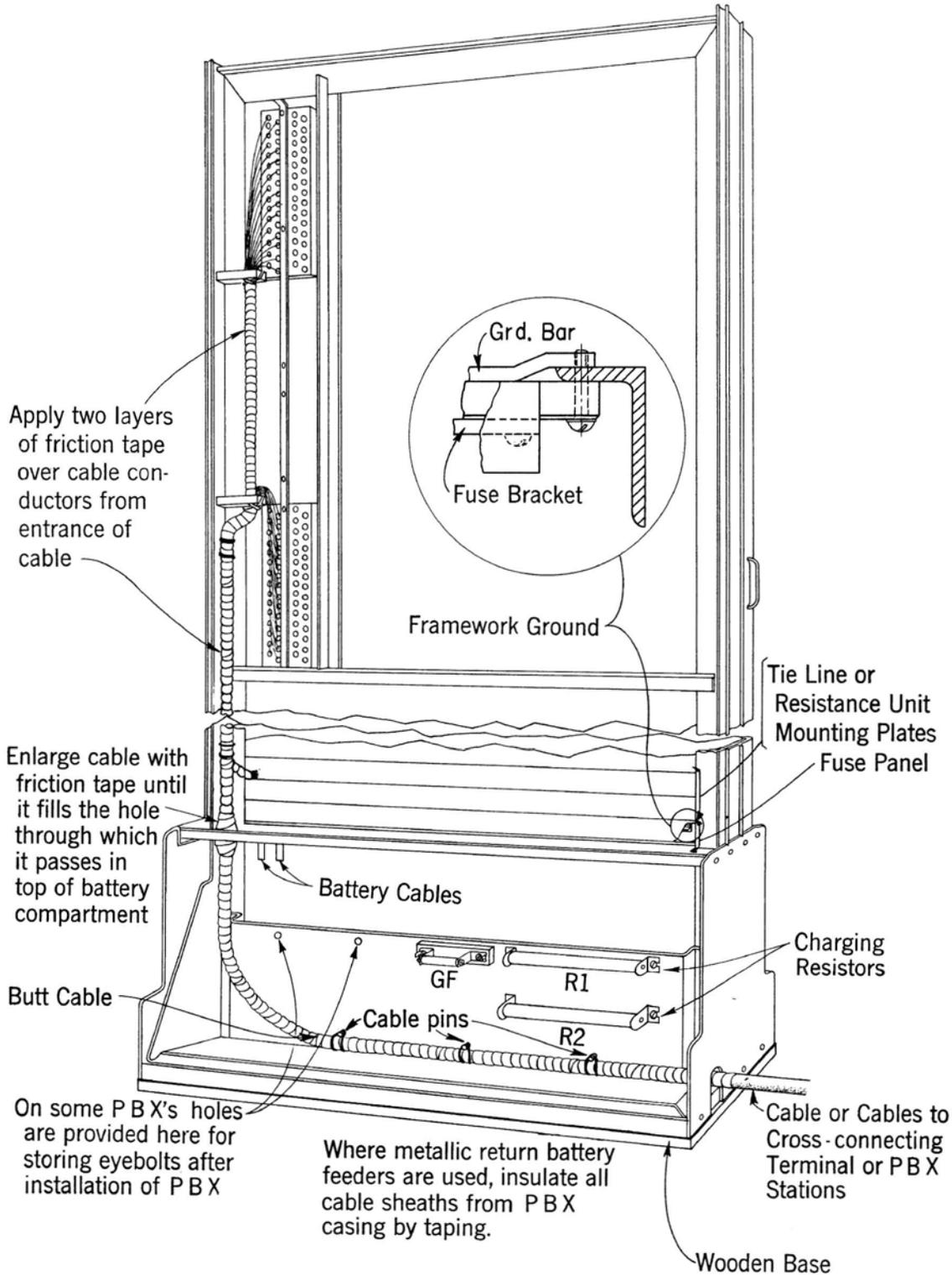
**Fig. 11 – Typical Cabling of PBX Where a Cross-Connecting Terminal is Provided – Cable Entrance at Bottom of PBX is Shown With Lead Covered Cable**
