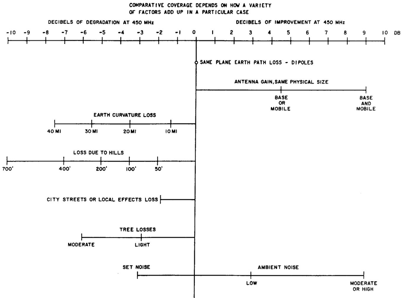
Fig. 1 -- Coverage Comparison -- 450 MHz Versus 150 MHz
