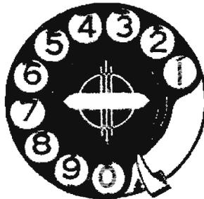
Dial with "Cutaway" Finger Plate
