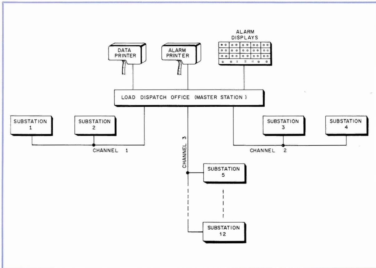
Figure 6. Substations throughout the power system's service area are supervised from the load-dispatch office at St. Petersburg. Microwave communication channels are shared with the existing "protective relaying" equipment and voice facilities.
