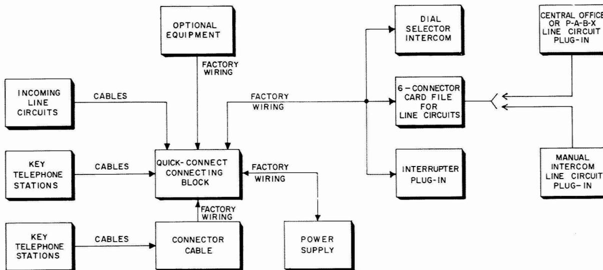
Figure 2. Interconnection of components in the 10A2 Key Telephone System.
