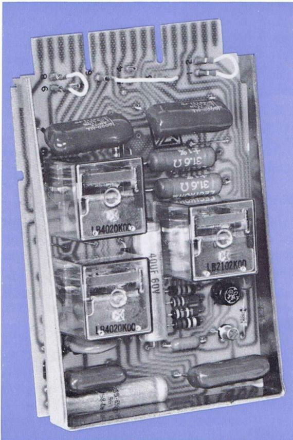
circuit permits an additional ringer to be placed ahead of the circuit, if needed, without danger of pre-trip. This was not possible with either the 10A or 10A1 line circuits.
