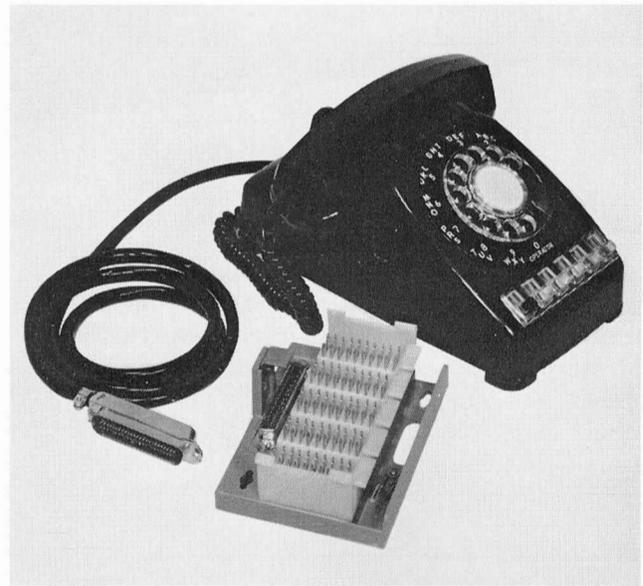
Figure 1. The 10A2 Key Telephone System, consisting of control equipment (left), and station equipment such as the Type 86 plug-ended key telephone and quick-connect terminal boxes (right), is engineered for fast installation and easy servicing.
