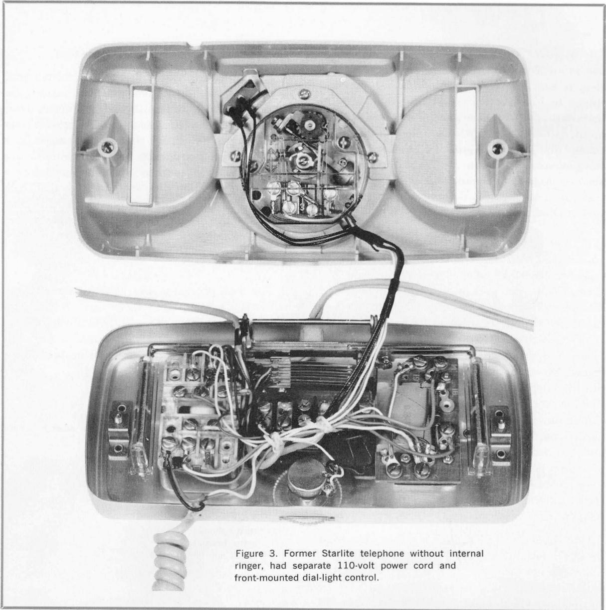
Figure 3. Former Starlite telephone without internal ringer, had separate 110-volt power cord and front-mounted dial-light control.
