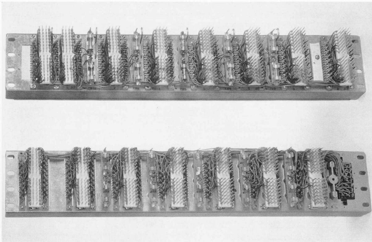
Figure 9. Rack mounted 15-line panel (top) and 13-line panel (bottom) viewed from the rear.
