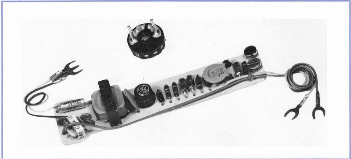
Figure 2. All amplifier components except the volume control are mounted on a semi-flexible board measuring only  $3\frac{7}{8}$  by  $\frac{3}{4}$  inches. (Shown actual size.)
