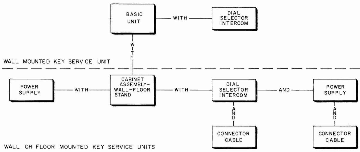
Figure 5. Eleven combinations of pre-wired key service components and two varieties of power supplies are available from the factory.
