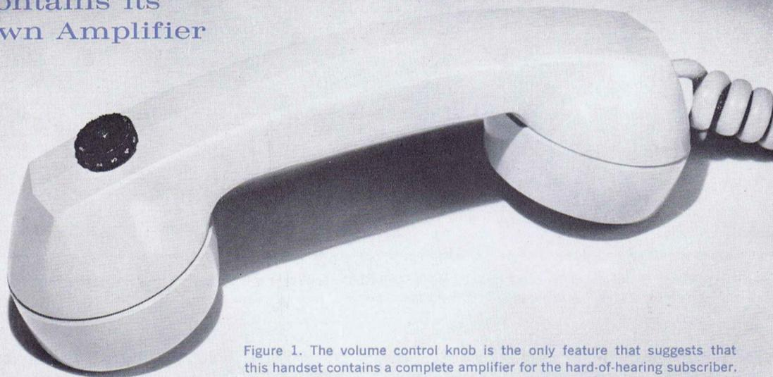
Figure 1. The volume control knob is the only feature that suggests that this handset contains a complete amplifier for the hard-of-hearing subscriber.
