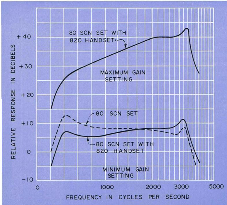
Frequency-response curves (Figures 6) show the performance on a two-mile loop of 26-gauge non-loaded cable. Increase of gain causes an increase in the high frequencies where most hearing deficiencies occur. However, at maximum output, the sound levels will not injure the user's ear; signal levels are limited by the overload characteristics of the amplifier and by the click-reducing characteristics of the silicon varistor across the receiver.
