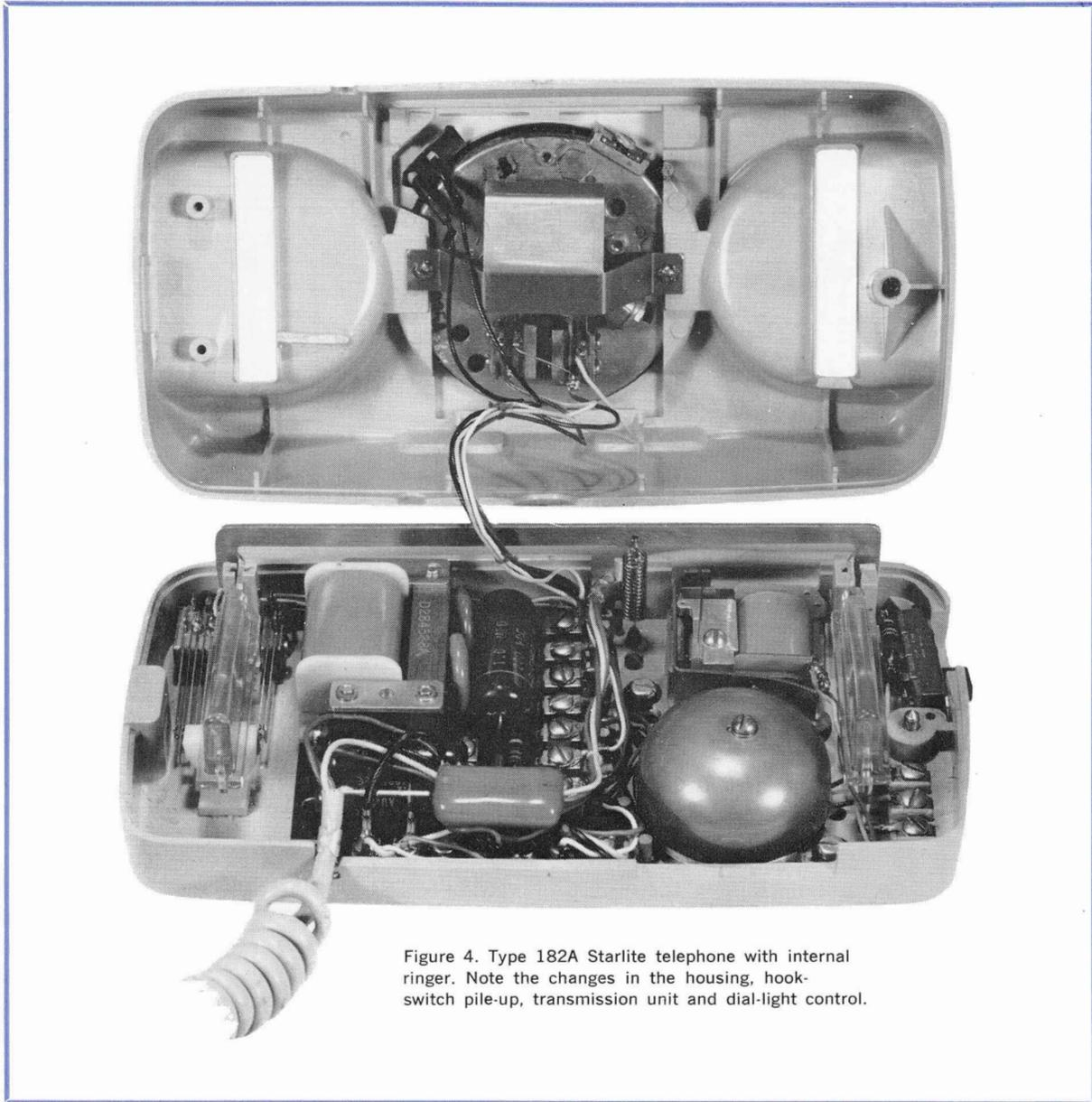
Figure 4. Type 182A Starlite telephone with internal ringer. Note the changes in the housing, hook-switch pile-up, transmission unit and dial-light control.
