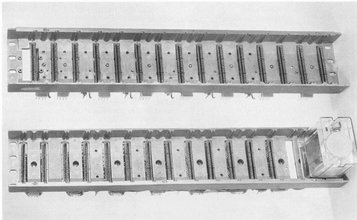
equipment—with the plug-in concept incorporated in all equipment. As a result, the AE 10A2 Key Telephone System reduces time consuming installation problems common to the older systems. The plug-ended telephone instruments, factory wired and equipped key service units, optional plug ended cables, and solderless quick-connect terminal blocks save installation time. Plug-in line cards, which are used on an “as required” basis, minimize the operating com-
