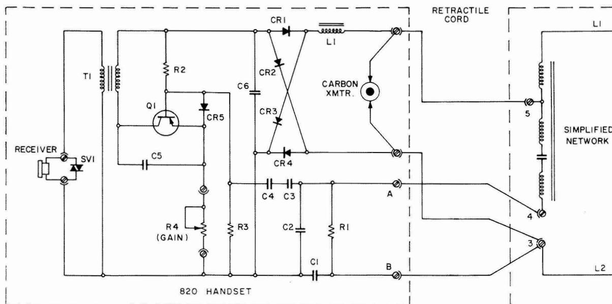
Figure 4. Diagram of the 820 Sound-Booster Handset, showing its relationship to the transmission network.
