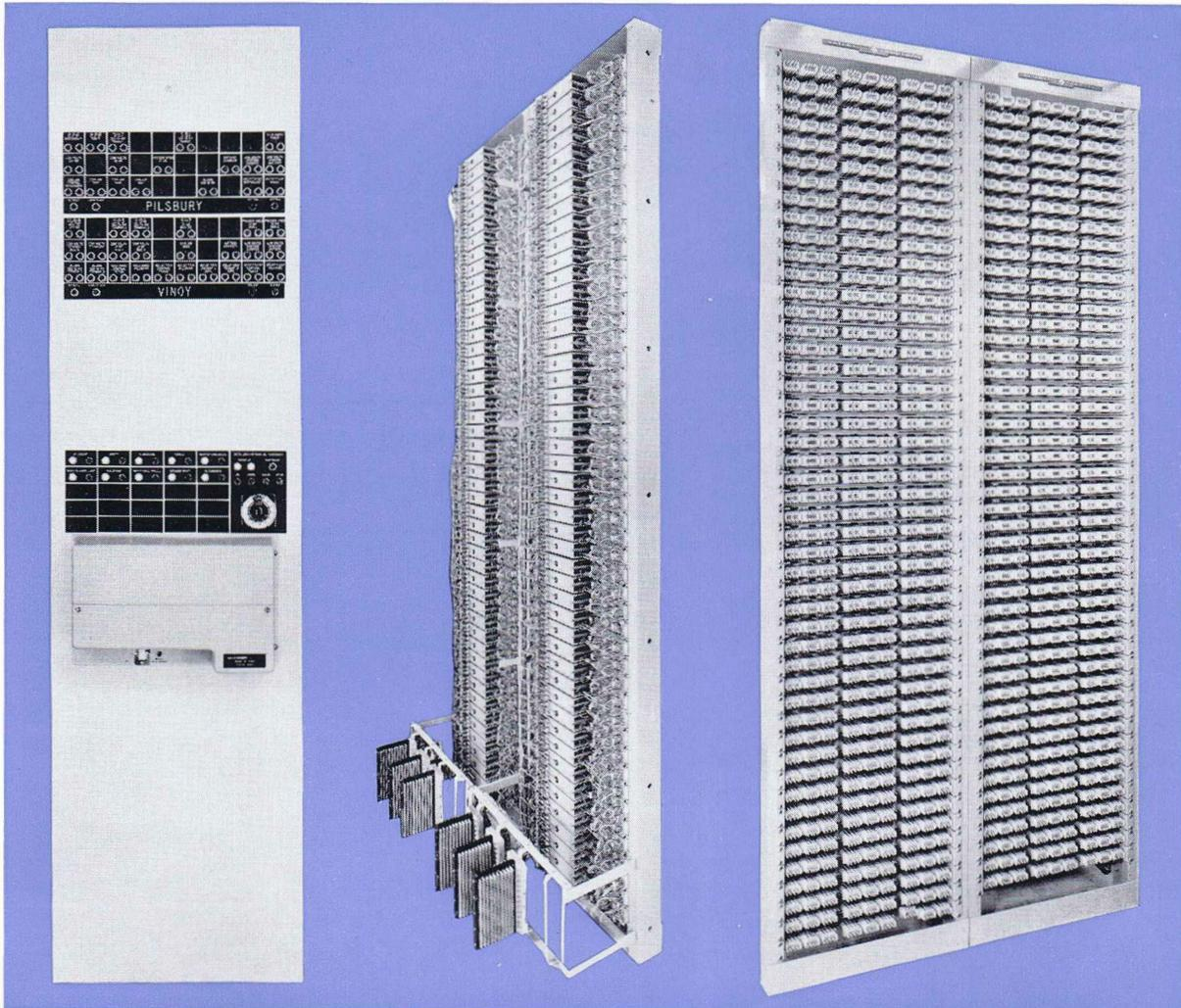
Figure 3. (Left) Display panel divided according to substations, each section having lamps for indication of alarms at a particular remote station. The status of each point is displayed by means of two lamps, one green for "alarm" and one red to indicate a "no alarm" status. A teletypewriter printer mounted at the bottom of the panel can write up to seventeen 16-column lines per second, permitting print-out of telemetered information without delaying other system operations.
