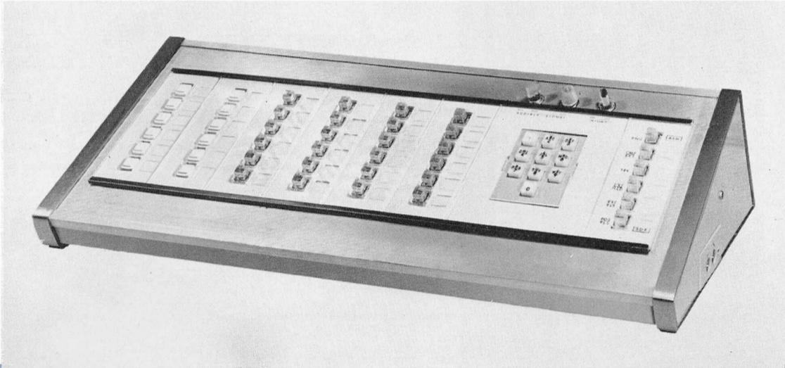
This 36-trunk turret for the Type 300 PABX provides an intermediate size between the 24-trunk desk turret and the 48-trunk floor console. Measuring 5 inches high, 10 inches deep, and 22 inches wide, the new turret is equipped for 24 trunks and is completely wired for 36 trunks. Six lamp strips, four key strips, and two dummy key strips (positions for future key strips) are pro-
