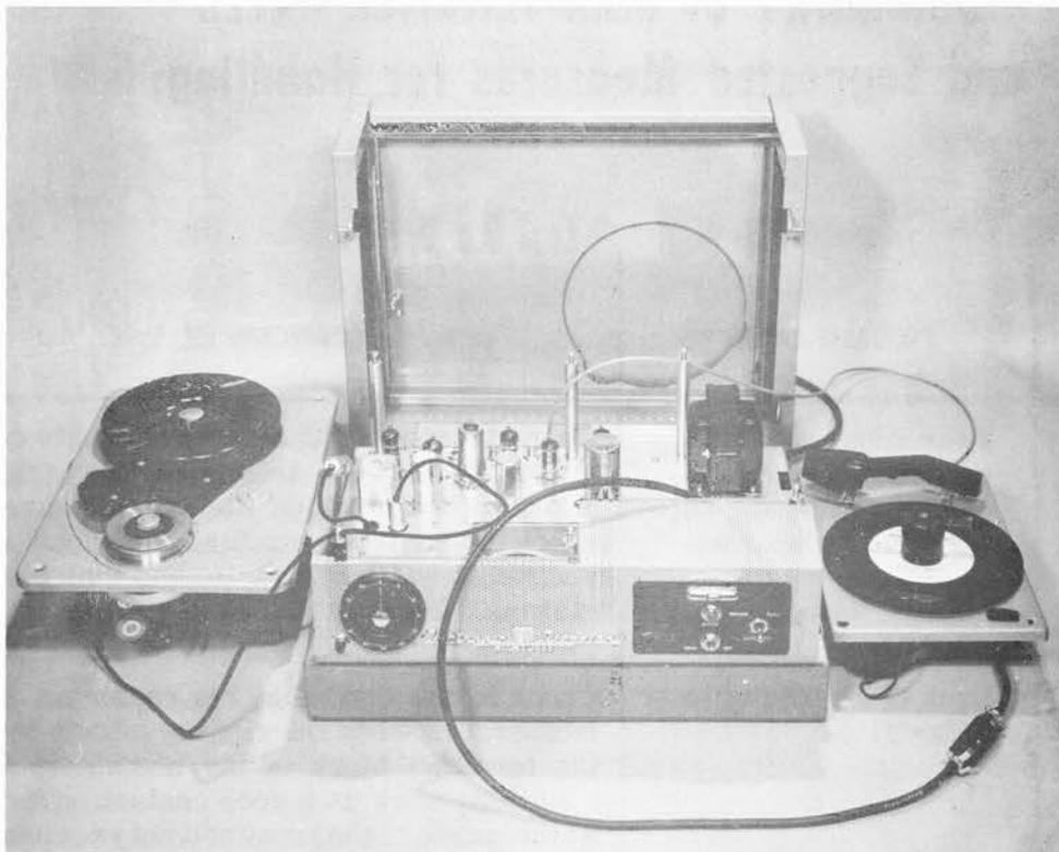
Photo shows chassis with wire recorder mechanism and record player mechanism removed and with test extension connector leads used to duplicate normal operating conditions.
