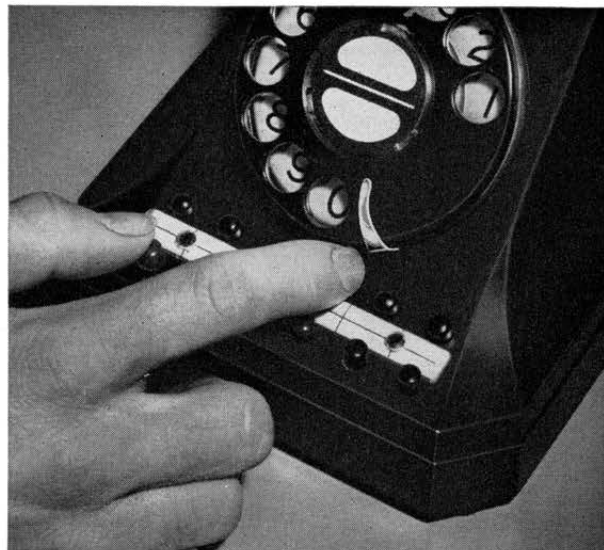
Operation of Push Buttons to Transfer a Call Buttons 1-5 Operate Station Signals for Inter-Communicating Buttons 6-7 Connect Telephone with an Outside Line Button 8 Holds an Outside Call while Ringing Another Station
