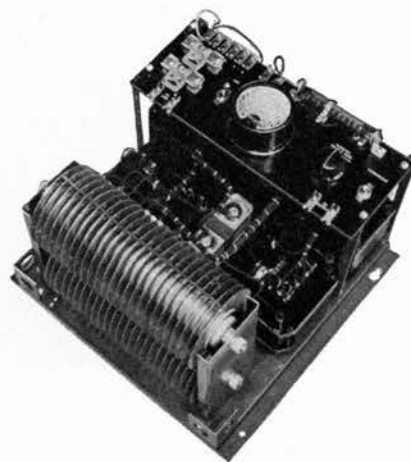
View of interior apparatus of the Raytheon Recticharger
