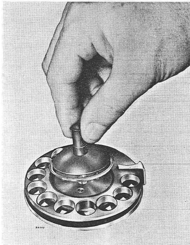
FIG. 18.—MOULDED BODY DIAL—REMOVAL OF LABEL PROTECTOR WITH EXTRACTOR NO. 29
