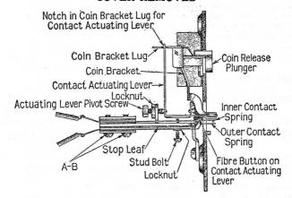
11. Adjusting contact actuating lever. With the armature in normal position the contact actuating lever should rest in bottom of the notch in lug on the coin bracket. If necessary to adjust remove coin mechanism (see Section 4, page 5) and bend lever carefully to right or left with finger until proper adjustment it secured. Make sure that lever slides smoothly on sides of notch when relay armature is operated to either "collect" or "return" positions.
