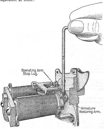
If the rocking fingers on the coin bracket are bent or twisted so that coins are not collected or refunded when stop lugs are properly adjusted replace collector and return for repairs.
