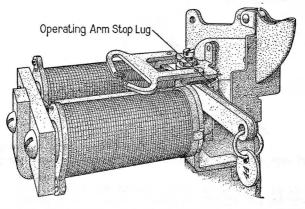
If necessary to obtain proper gauge adjustment between stop lugs and frame, bend lugs carefully with #143 Tool or equivalent as below:
