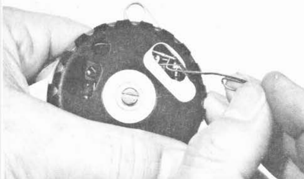
Figure 18. Adjusting Bias Spring in P1A Ringer
