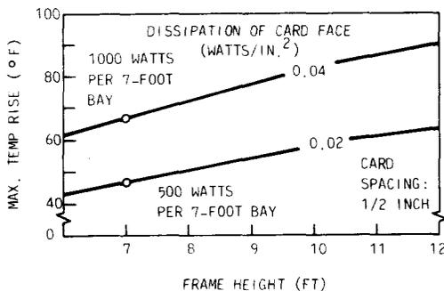
Fig. 2—Temperature Rise in Free Convection for Equipment of Different Height
