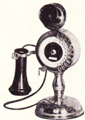
The common battery desk telephone of 1907 incorporated many improvements in design. Made of nickel plate, very elegant and imposing.
