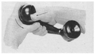
Fig. 2 To Remove Mouthpiece, Turn Metal Ring in a Counter-Clockwise Direction Holding Moulded Piece with Thumb
