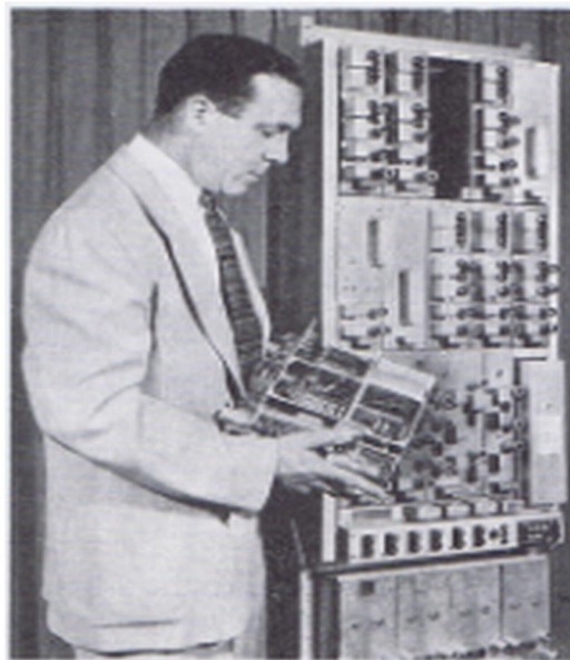
Fig. 8. Type- N terminal equipped with schedule A channel unit and plates. Engineer inspecting schedule C unit
