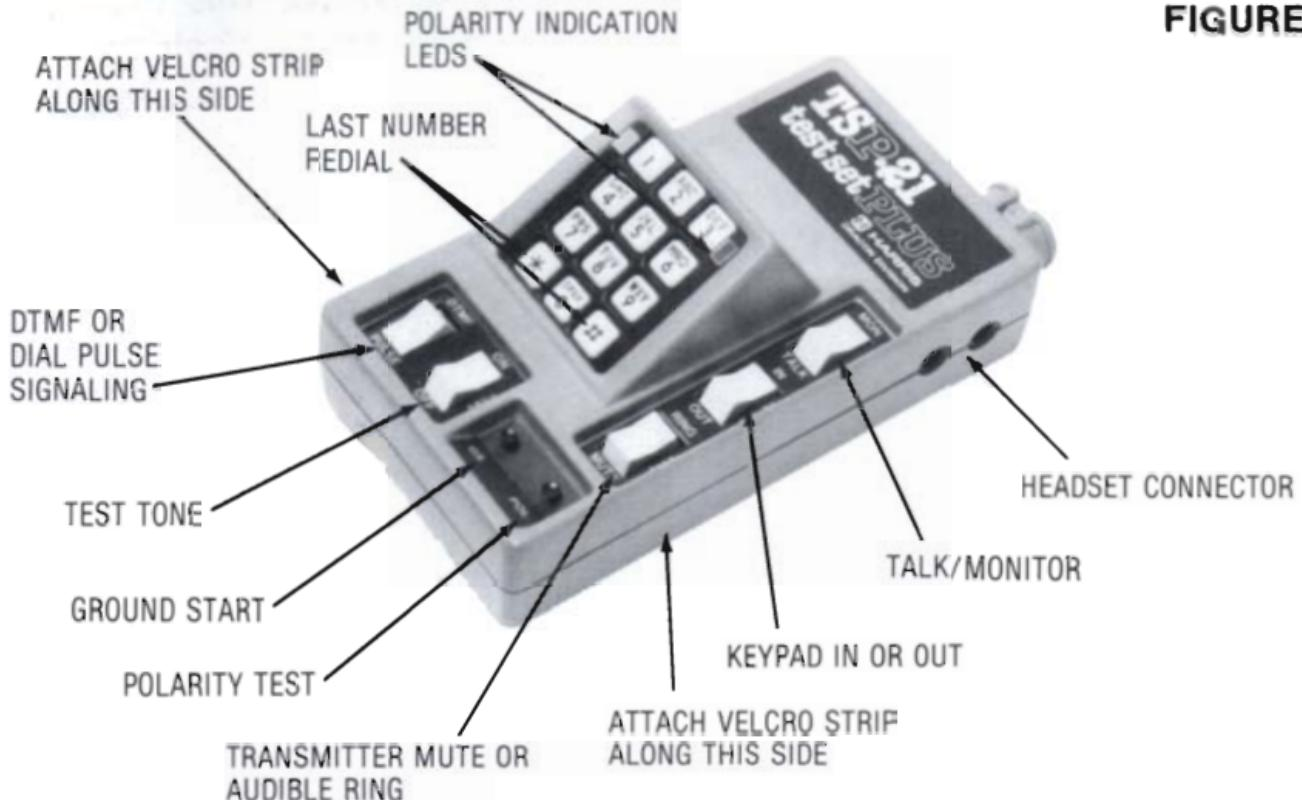
keypad bezel to check line polarity. Pressing the POL (polarity) button when the TALK/MON switch is set to "MON", and the Test Set is connected to a telephone line or battery source, will cause one of the LEDs to light. The yellow LED will light if the red test lead is connected to the ring (negative) side of the line and black test lead is connected to the tip (positive) side of the line. If the position of the test leads is reversed, the red LED will light.
