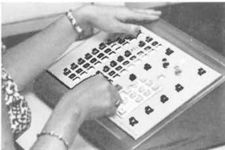
Small, modern desk consoles can replace switchboards. One of two types now in use is shown above.
