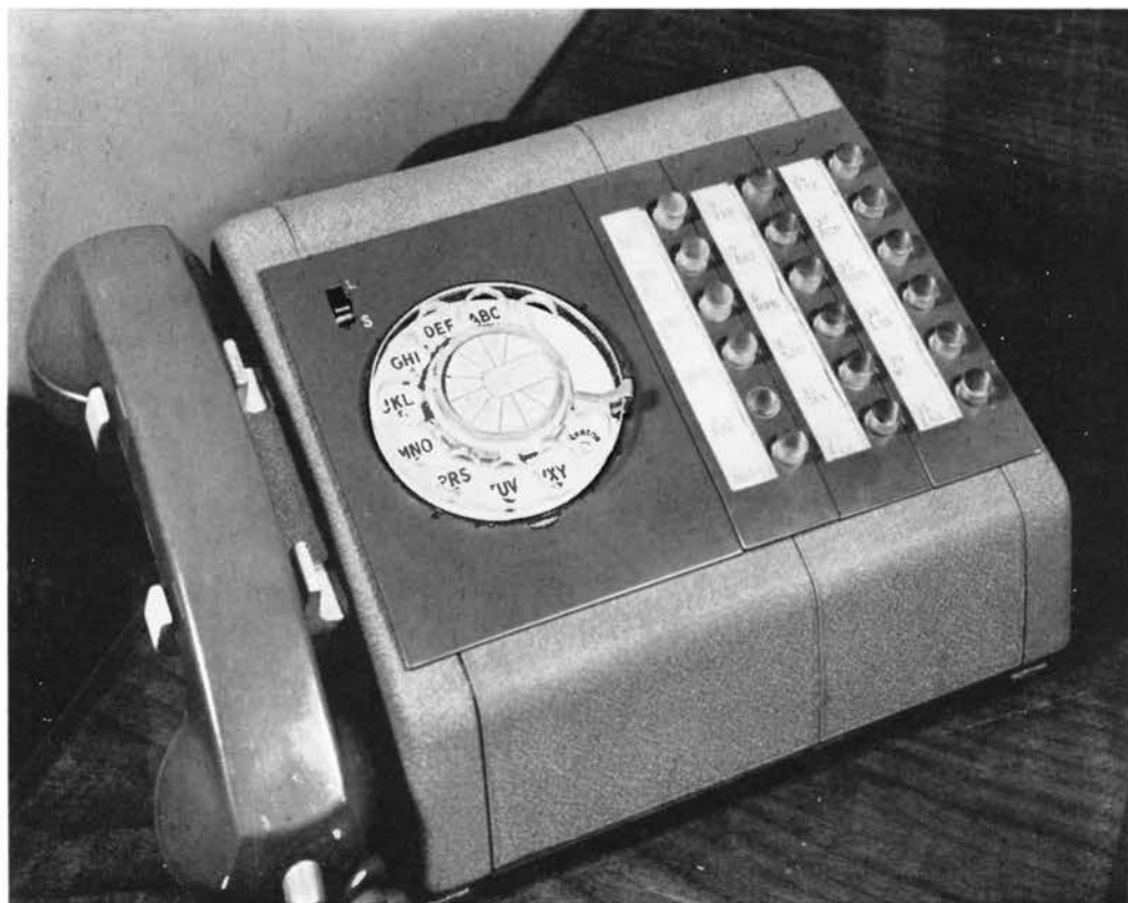
A modular console with 18 push-buttons
