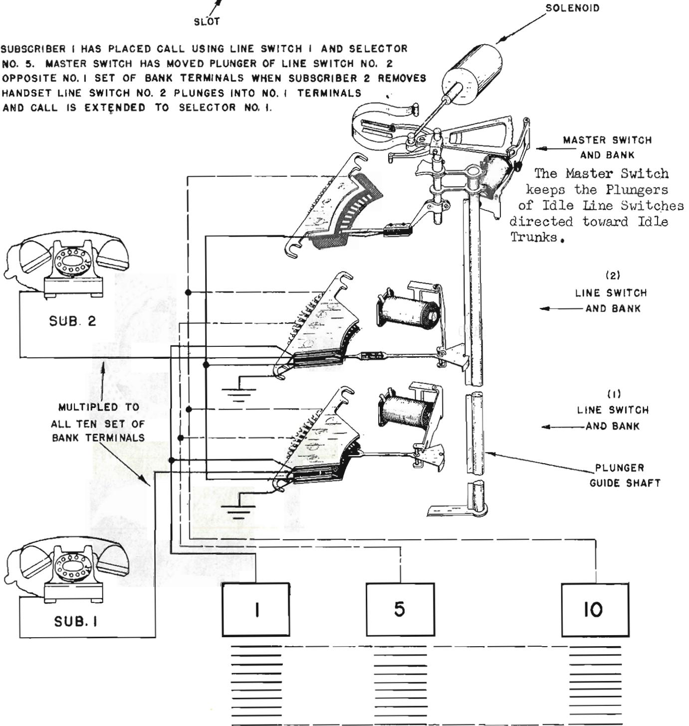
The Master Switch keeps the Plungers of Idle Line Switches directed toward Idle Trunks.
