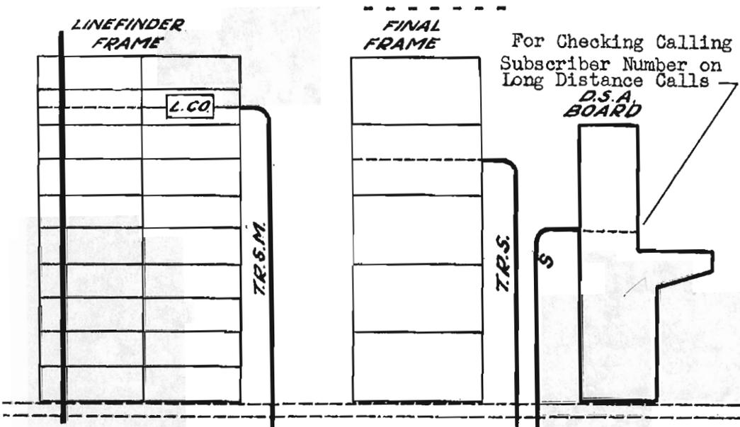
Cabling Between Distributing Frames and Panel Dial Switching Frames
