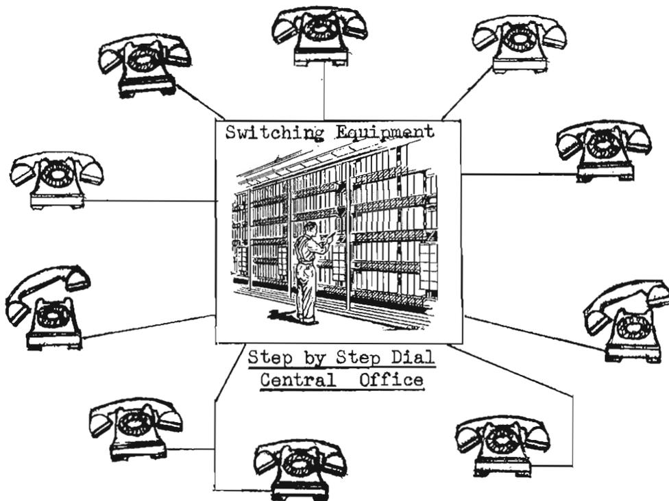
Subscriber Line - A 2-wire Path between a Subset (Telephone) and the Switching Equipment in the Central Office.
