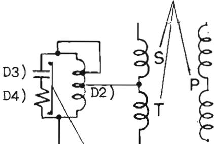
D2) Sidetone Balance Coil - Maintains a constant balance (flat response) over the voice-frequency range.
