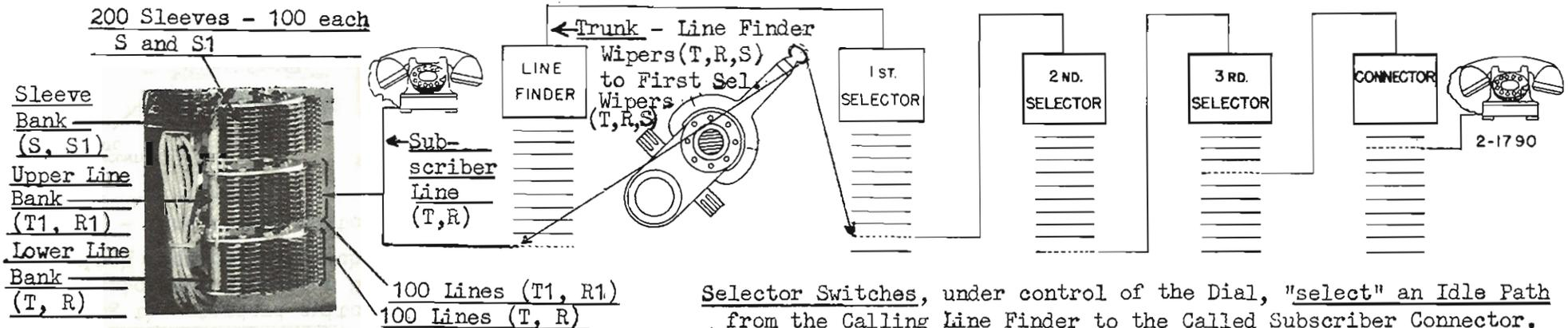
Selector Switches, under control of the Dial, "select" an Idle Path from the Calling Line Finder to the Called Subscriber Connector. The Connector Switch, under control of the Dial, "finds" the Called Subscriber Line.
