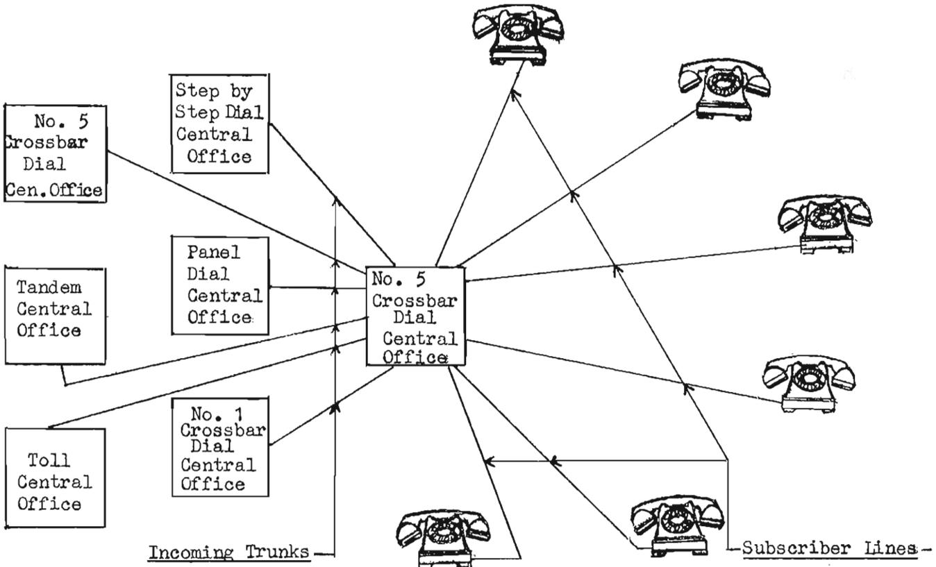
Tandem Office - A Central Office used as an intermediate Switching Point for traffic between other Central Offices.
