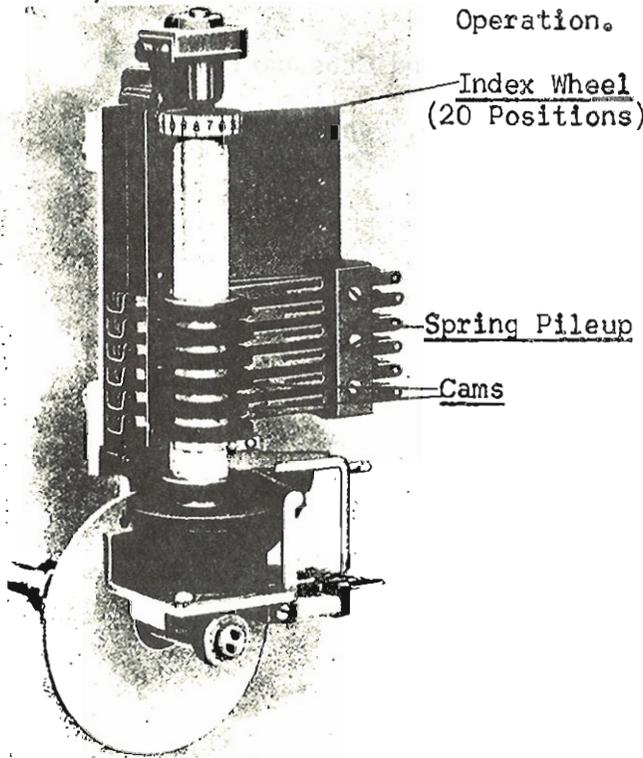
The Register controls Selector and Final Switch operation (On a Revertive Pulse basis) as it restores to normal, after being advanced by Dial Pulses to the position representing the Digit Dialed.
