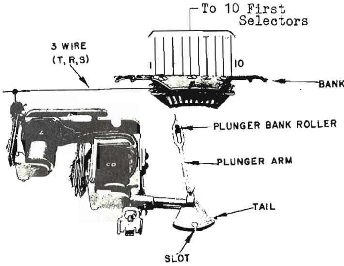
The expensive Switch used for each Subscriber Line in early Strowger Exchanges was replaced by a smaller and more economical Plunger Type Line Switch, developed by A. E. Keith, and first used in 1907. Thus each Subscriber Line terminated in one of these Line Switches, which operated to connect that Line to an Idle First Selector Switch when the Calling Subscriber removed his Handset.
