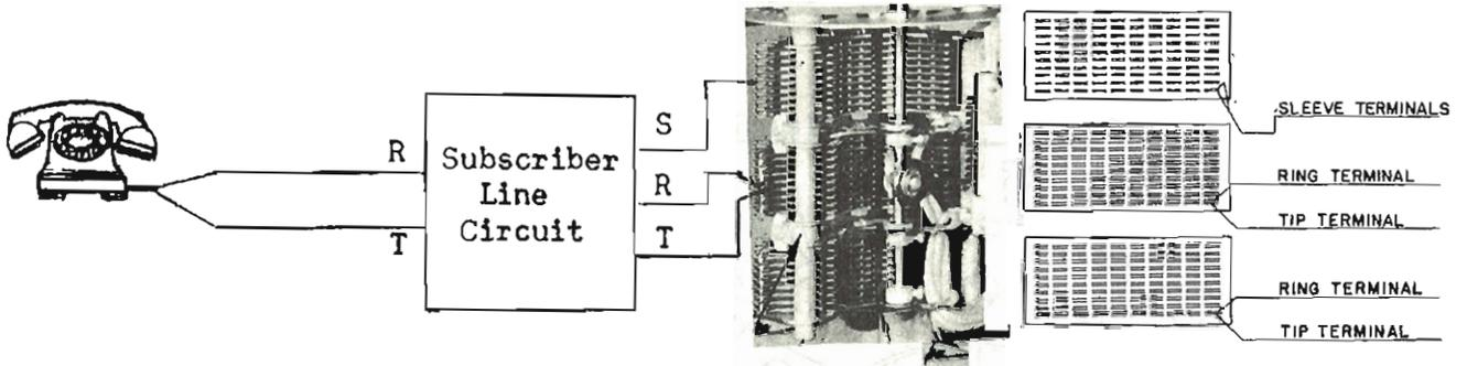
3) A SET OF MULTIPLE BANK STRIPS in the PANEL Dial System
