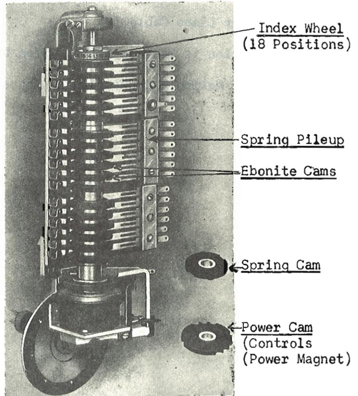
As the Sequence Switch rotates only in one direction, it always opens and closes the circuits wired to its contacts in the same order or "sequence."
