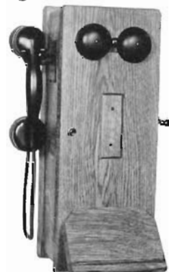
Typical Magneto Telephone, After Conversion
