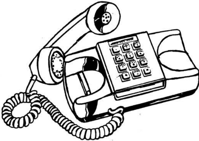
Type 182 Desk Touch Calling Telephone or Push buttons with Universal Dialing Keypad (Rotary Dial Version not shown)
