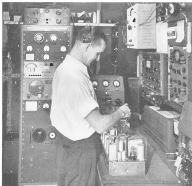
Mobile telephone service presented the Shops organization with a big new post-war task: gearing up for complex repair jobs. This receiving set is being fixed in a copper shielded booth in one of the shops
