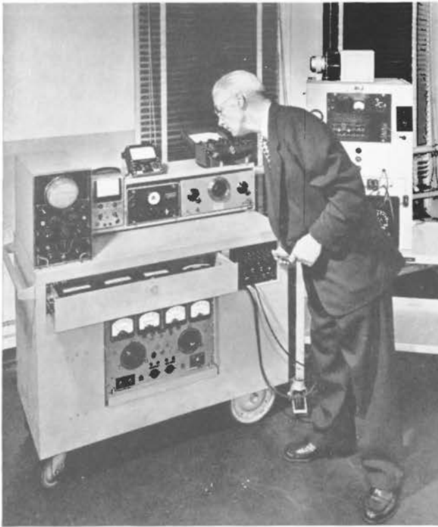
A miniature laboratory on wheels, for use in testing test sets, gets a final check in the Engineer of Shops laboratory
