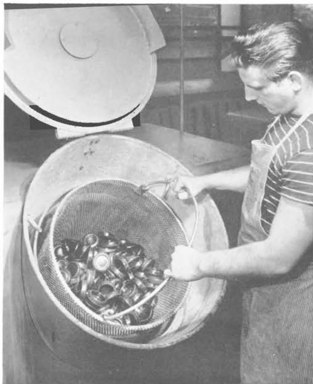
This machine automatically washes telephone parts at 160 degrees and then dries them
