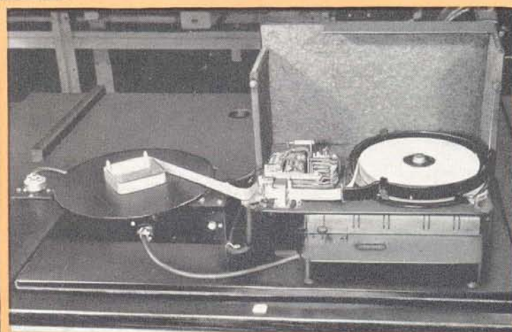
S.A.T.T. Tape Perforators. Tapes from these machines may be used to prepare conventional toll tickets, or used with automatic punch card billing procedures.
