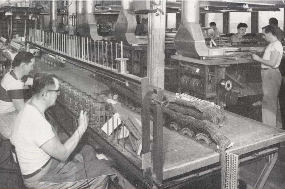
above: The Strowger switch bank multiple is designed and constructed for maximum durability and flexibility. Twisted pairs avoid crosstalk, and soldered connections make for permanence.
