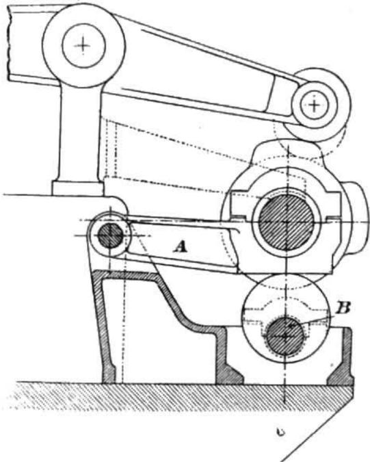
rockers. This invention has for its object a simple means of effecting this movement. The cam shaft bearings are mounted on rocking arms A, and an eccentric B is used to advance or withdraw the cam shaft.—February 5th, 1920.
