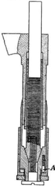
after compensating wear of the screw, the graduated thimble is attached to the stem of the measuring screw by means of a tapered joint, as shown. The thimble is made in two parts, and the usual ratchet stop A introduced between the two parts.—February 5th, 1920.
