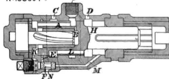
and passes to the passages A, and so to the rear end face of the piston H, thereby forcing it to the right. At the same time air passes by ports B to the hollow interior of the piston H and assists in propelling it. The incoming air also enters the passage
